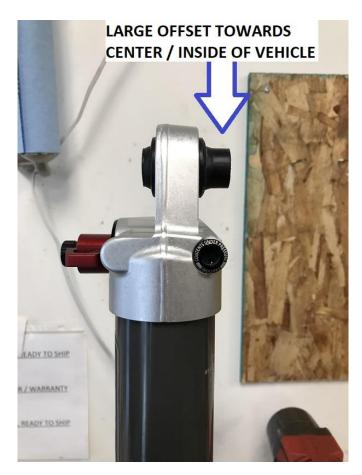
4) Be sure to orient the shock body so the reservoir is positioned towards the rear and the adjuster faces out. Torque the upper bolt to 100 ft-lbs (135 N.m).
