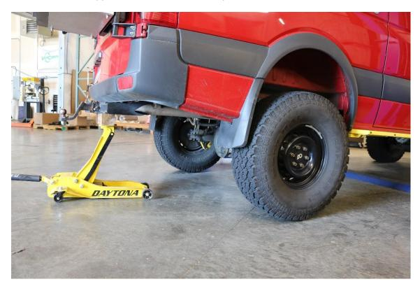
2) Note the shocks are left and right specific, refer to the part number etched on the shock body to ensure they are installed on the correct side.
