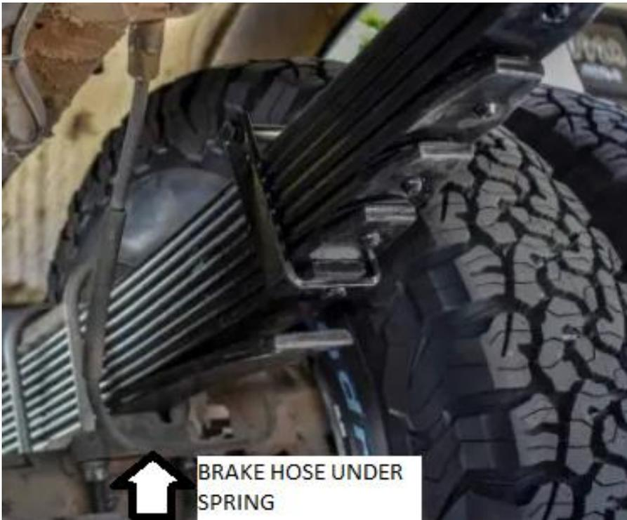
14) Once the springs are rotated into position. Install the forward spring bolt in the spring hanger slightly, install one of the provided washers between the spring and spring hanger. Push the bolt through the washer and into the spring. Install the second washer between the spring and hanger and push the bolt all the way through. Install the nut but do not tighten at this time.
