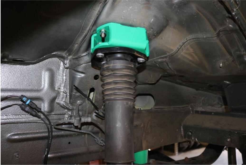
61) With all bolts installed and snug, torque to 21 ft-lbs (28 N.m)
