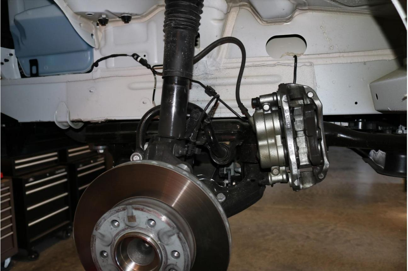
23) Raise the lower control arm about 3/8" (10mm) to remove tension from the strut. Use a 21mm socket to remove the 2 bolts securing the strut to the steering knuckle.
