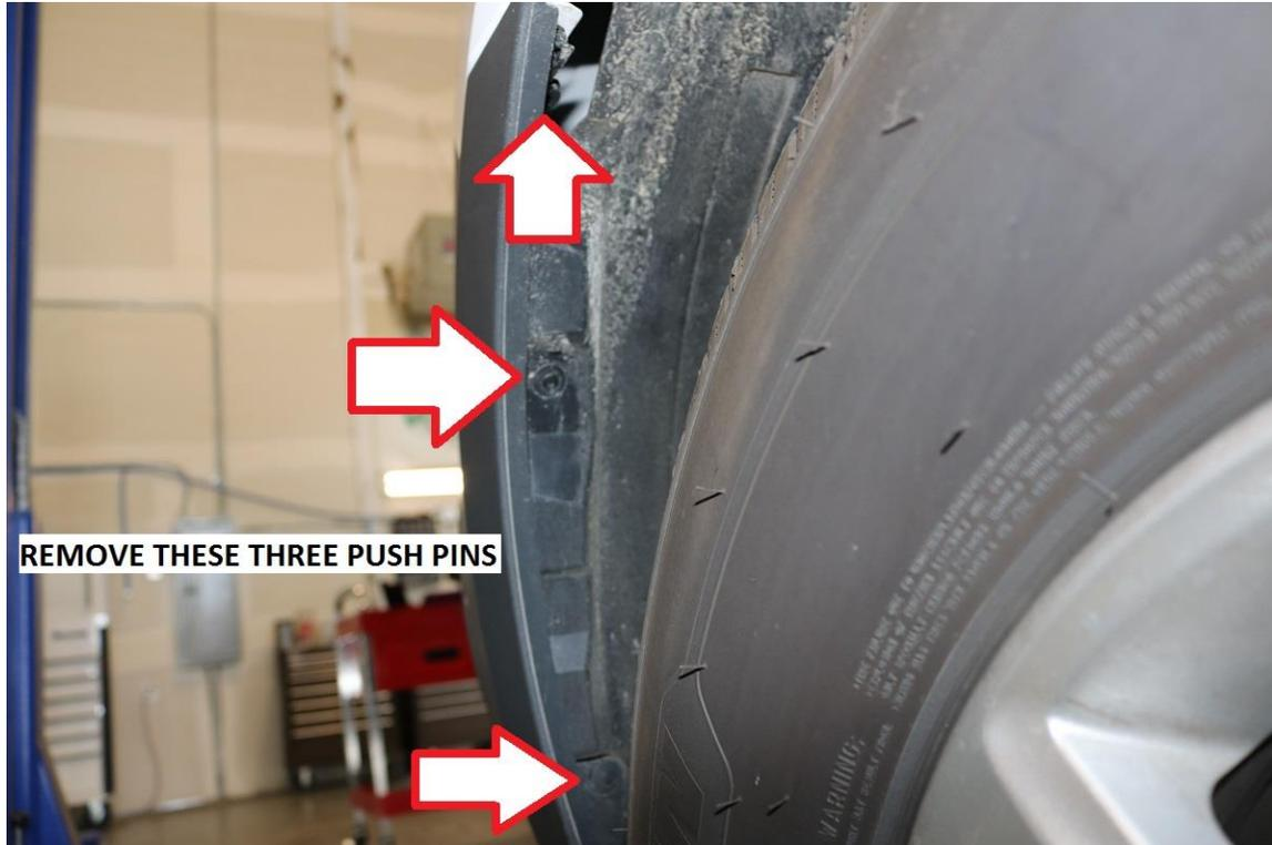
15) Locate and remove the three plastic nuts securing the front half of the inner fender well liner to the chassis. Use a 10mm socket for removal.
