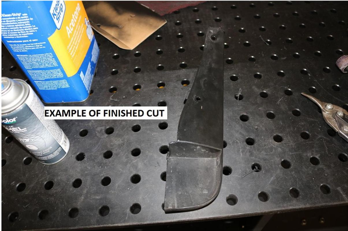
85) Mark a line at the bottom of the push pin mounting hole shown below. This is the bottom push pin mounting hole on the outside lip of the front bumper cover.
