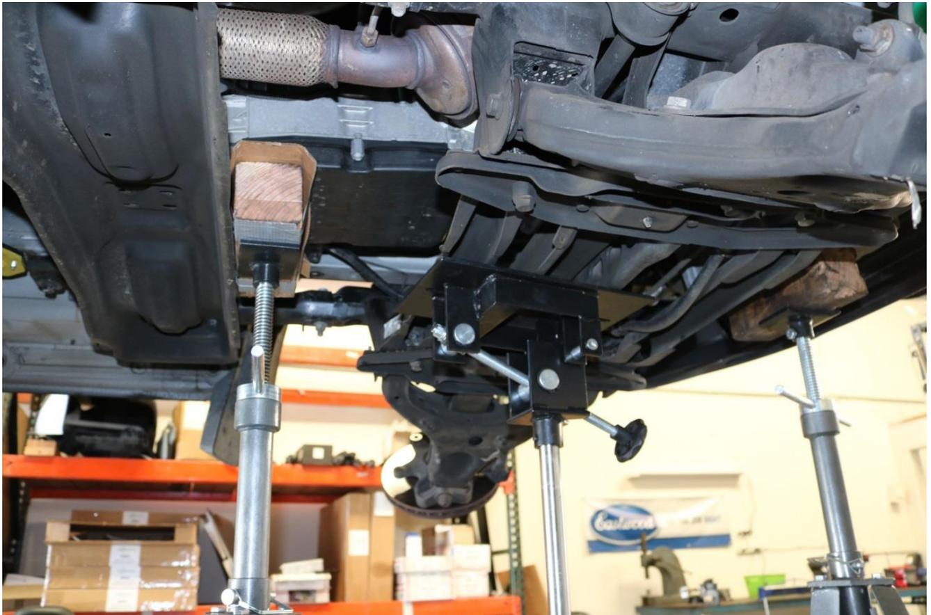
33) Remove the two transmission mount bolts shown below. Use a 16mm socket for removal.
