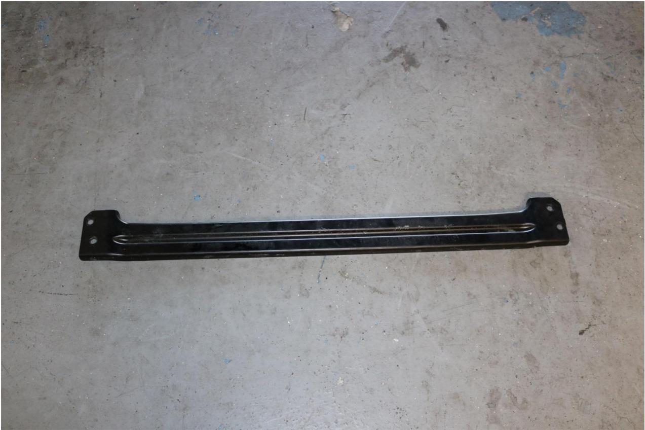
4) Remove the leaf spring skid plate by removing the 4 bolts securing it to the vehicle. Use a 13mm socket or wrench for removal.
