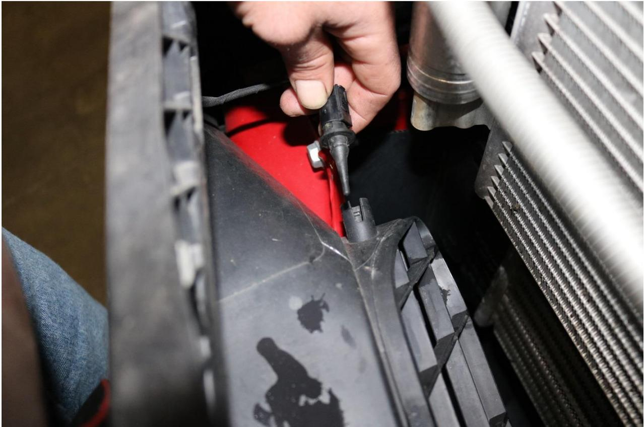
15) If the vehicle is equipped with fog lamps, disconnect the wiring at the lamps in each corner of the bumper
