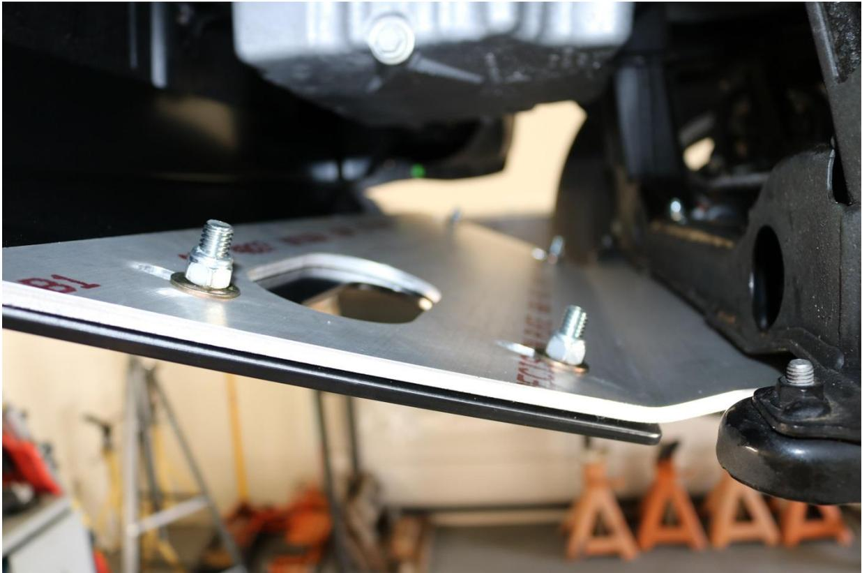
37) Align the front mounting holes and attach the front plate to the vehicle using the factory leaf spring skid plate bolts removed in step 4.
