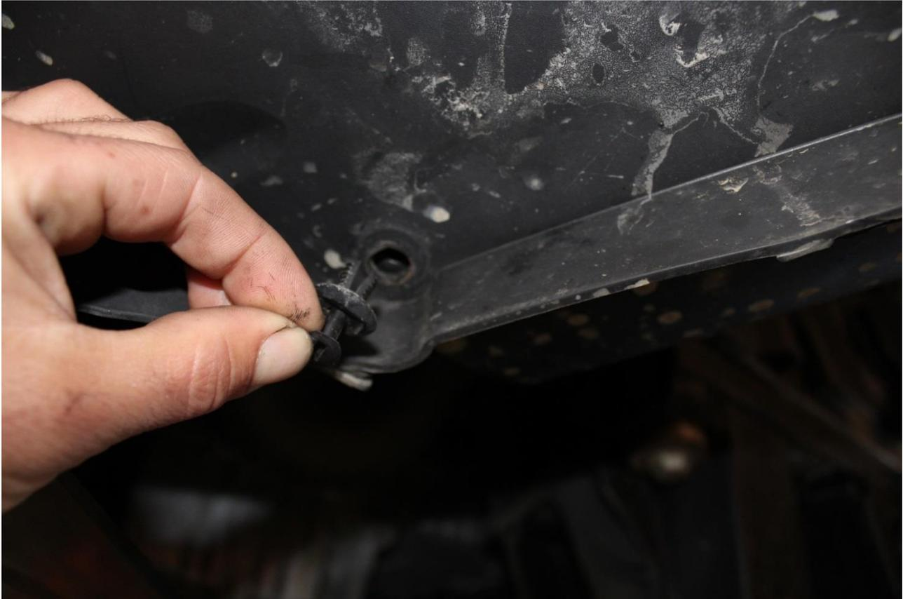
10) Next, on the inside of the fender well, remove the three push pin fasteners near the outer lip of the bumper cover.
