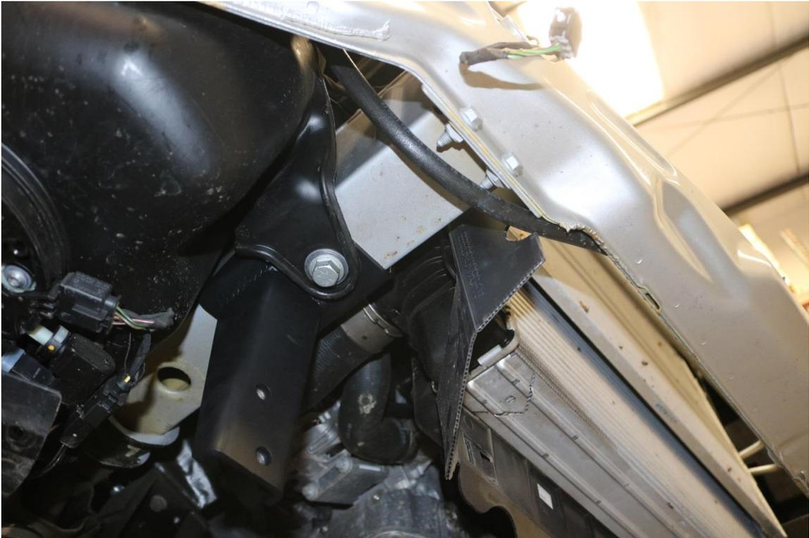
31) On the driver (left hand) side of the vehicle, locate the threaded hole on the bottom side of the “frame rail” and install the overrun mount using the M12-1.50 x 35mm long bolt provided in the kit. Use a washer under the bolt head and snug so the bracket is sitting flush on the bottom of the chassis.
