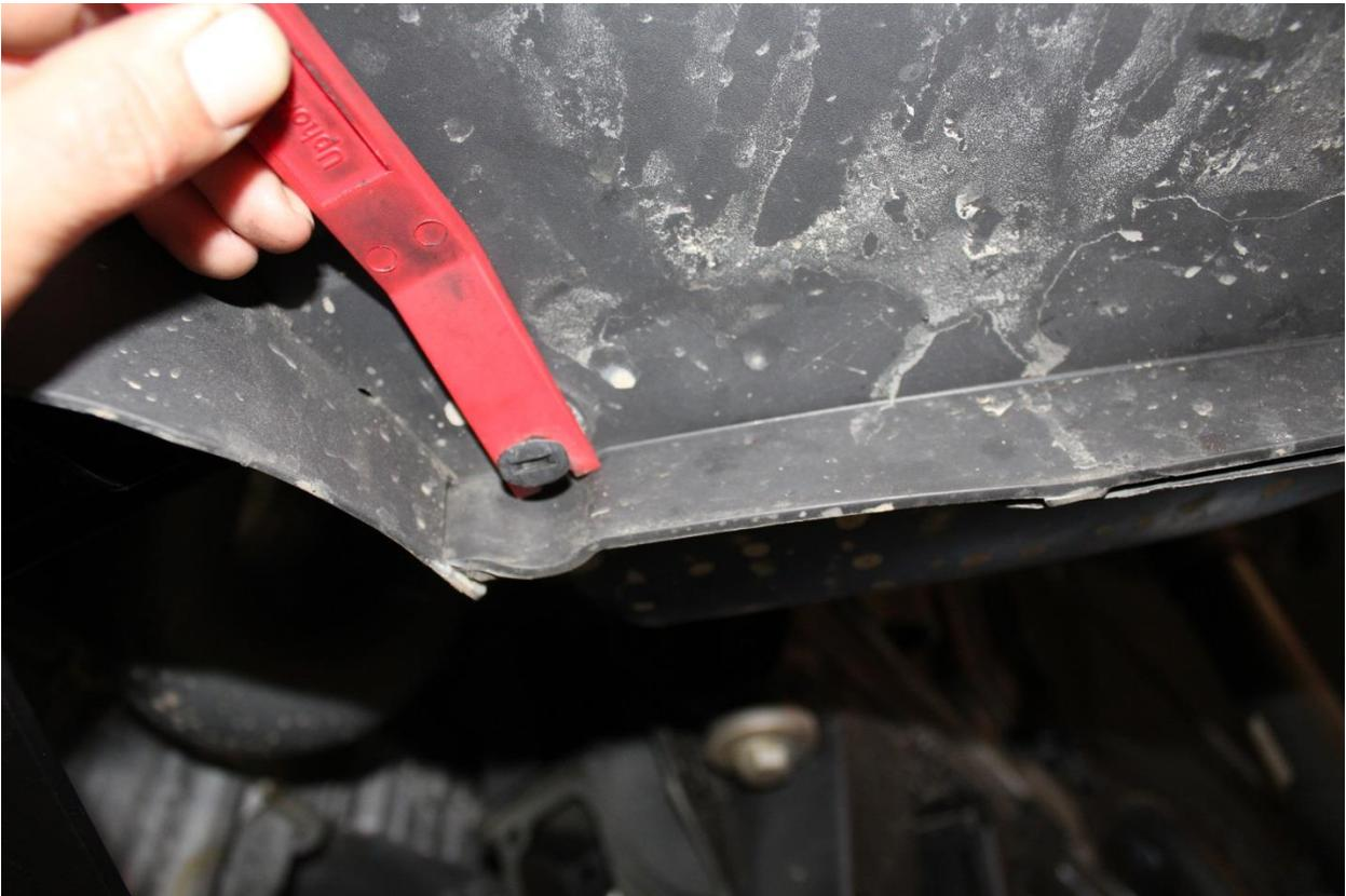
9) Using the same automotive trim removal tool, pry up under the head of the push pin body to fully remove the fastener. Remove these from both sides of the vehicle.
