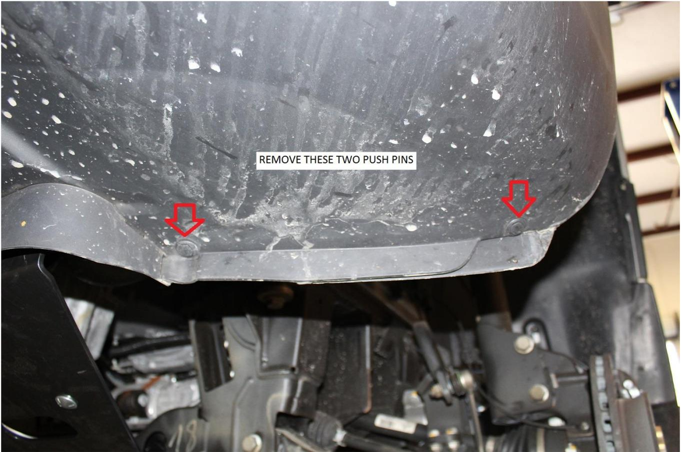
8) Next, using an automotive trim removal tool, pull up the head of the push pin.
