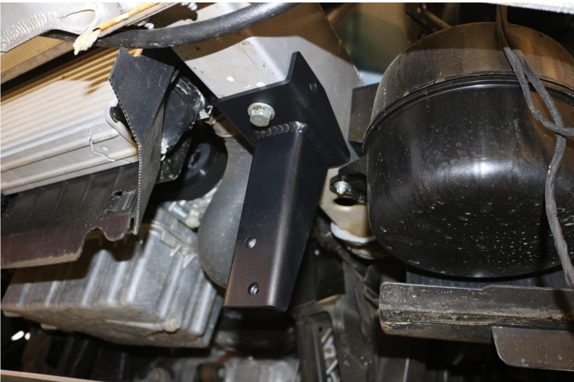
32) Using the Overrun bracket as a guide, drill the rear vertical mounting hole using a 1/2" (13mm) drill bit. See image below for reference.
