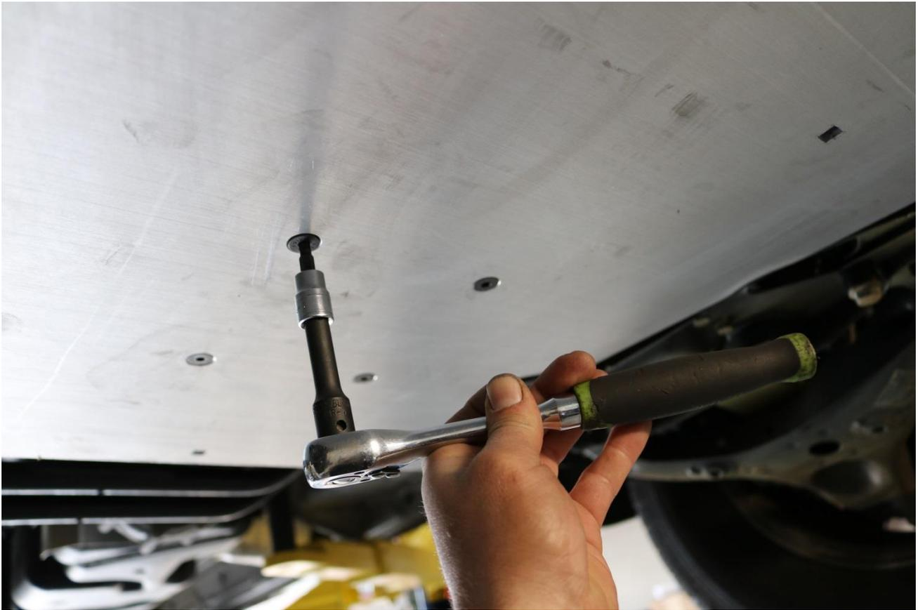
22) Install the 401001-05 front spacers. This is the shorter spacer. Install by placing the spacer in the access hole in the front cross member and sliding it over to line up with the mounting hole in the skid plate and cross member.
