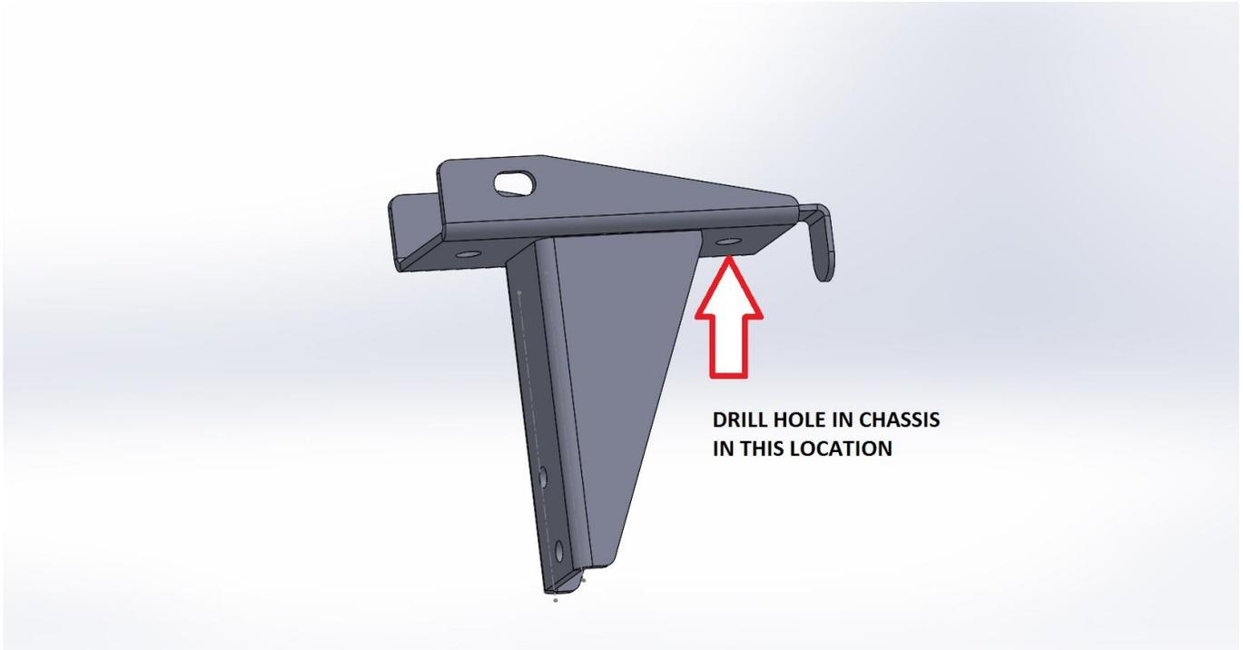
33) Install the included nut tab with the tab pointed downward through the hole in the chassis just behind the overrun bracket. See image below for reference.
