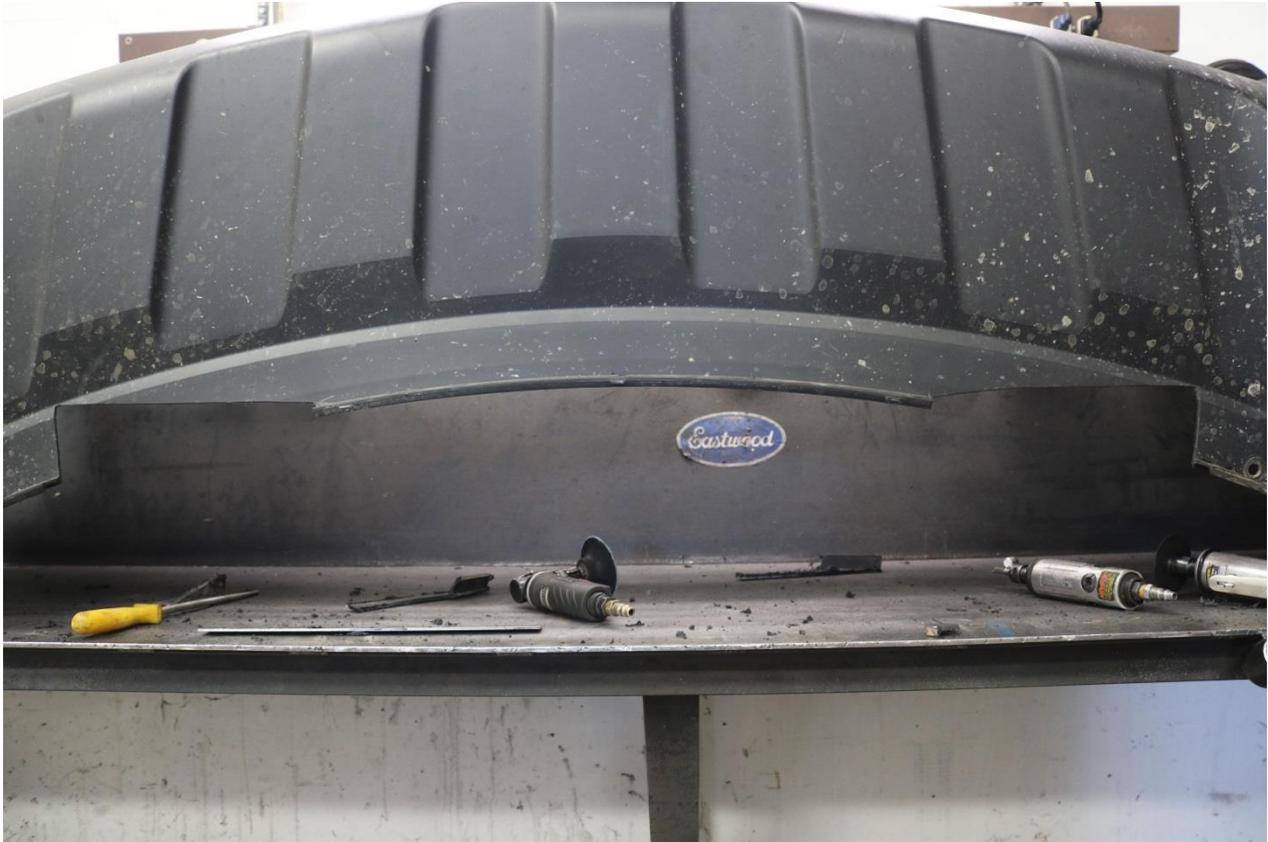
44) Test fit the trimmed bumper on the vehicle. Trim further if needed for the bumper to re-install smoothly.
