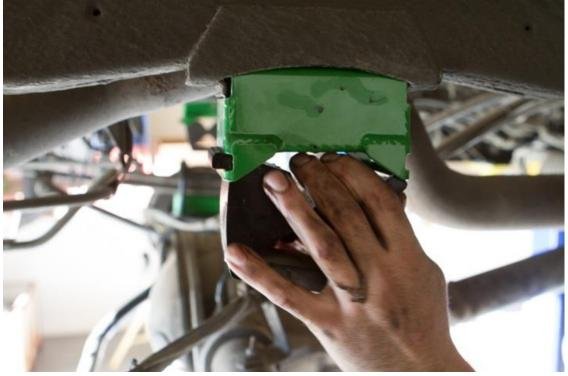
28) Once the second side is started, a screw driver, some wiggling and some additional lubricant will be needed to get the bump stop fully seated in the bracket.
