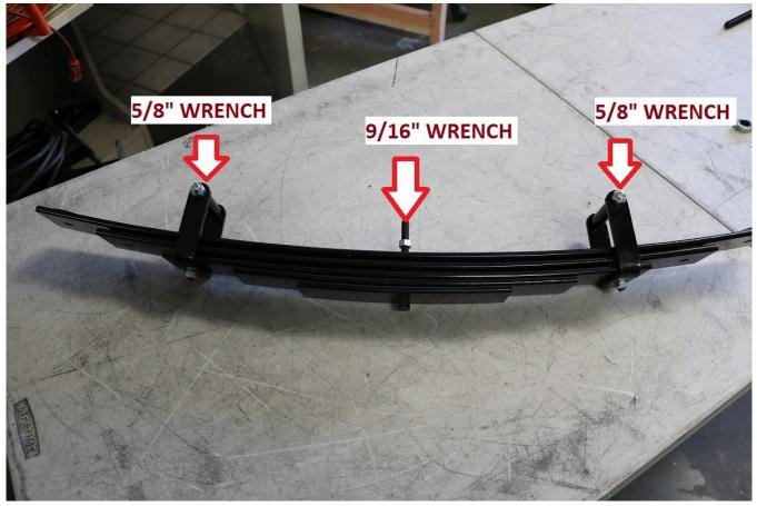
16) Assemble the leaf pack as shown below. Note, a 3 leaf installation is shown here. For the full lift kit installation, install all 5 leaf springs.
