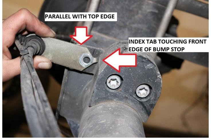
35) We have found it easiest to take the bump stop bracket to a work table or drill press to drill the hole.
