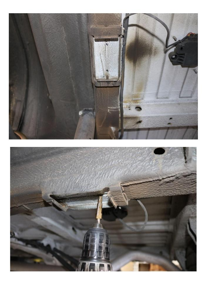
24) With both holes drilled, position the bump stop drop bracket in place and secure it to the chassis using the 5/16-18 x 1" long thread cutting screws included with the kit. Use a nut driver or drill with a ¼" bit adapter and a ½" socket to install the screw. Try to keep the drill / driver as straight as possible when cutting the threads.
