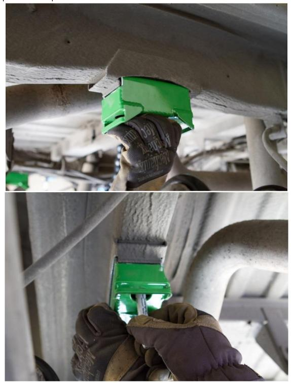
23) Since there is groove where the mounting holes land, a step drill will need to be used for drilling. Center punch the hole locations and drill with a step drill bit to a diameter of ¼" (7mm).
