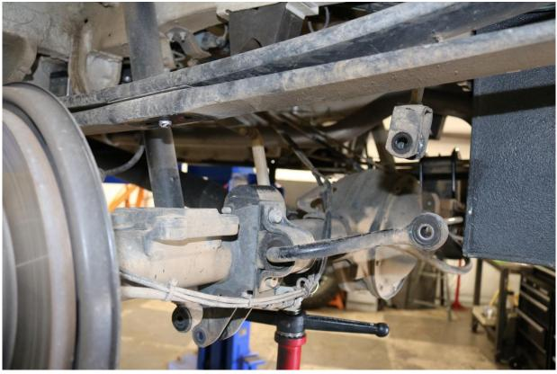
12) Remove the leaf spring center pin. Use a 16mm socket / wrench to remove the nut securing the center pin. Note; in some instances the center pin may need to be held with a pair of vise-grips as shown below.
