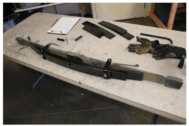
17) Install the leaf pack back into the vehicle. Align the center pin with the main leaf spring and use some C-clamps to preload the springs into place. Do not use the center pin nut itself to suck the leaf springs into place as the threads can be easily strip in that situation..
