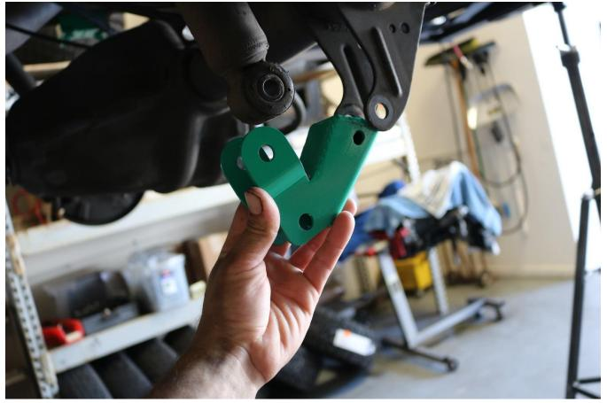
31) Install M8-1.25 x 65mm long bolt provided as shown above to locate bracket in place. Use a washer under the bolt head.
