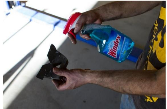
27) Install bump stop into the drop bracket. Install one edge at a time. Bend the bump stop in the middle to get the second side started. Installation can be tricky as the bump stops fit very tightly both in the factory location and in the drop brackets.
