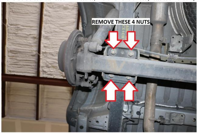
9) Remove the U-bolts and slowly lower the axle approximately 2.0" (60MM) or until the lift block can be placed between the axle and the leaf spring.
