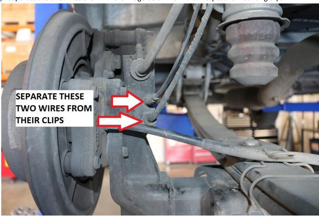
7) Cut the two zip ties securing the E-brake cable to the rear axle as shown below. Also, support the rear axle.
