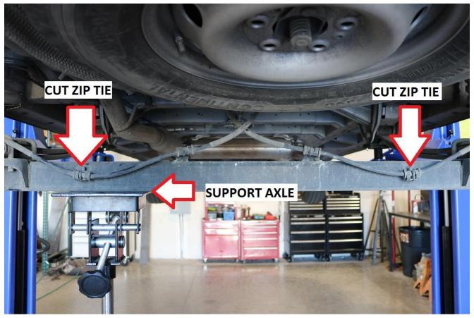
8) Remove the U-bolt nuts. Use a 22mm socket / wrench for removal. See photos below for clarity.
