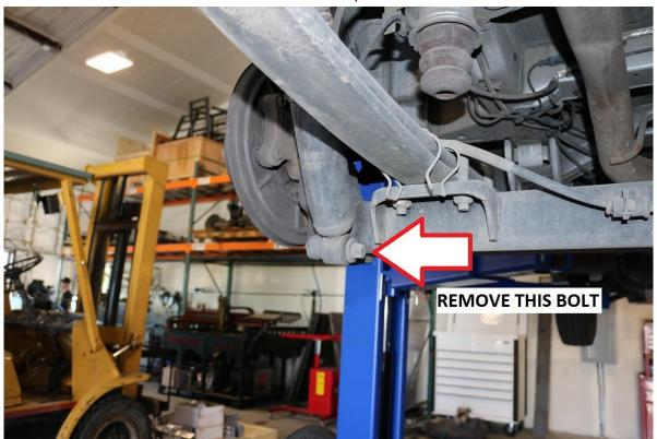
5) Remove the upper shock bolt and remove the shock from the vehicle.
