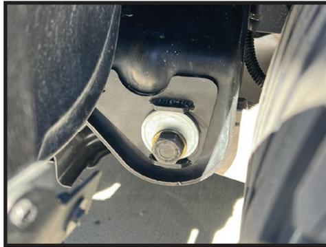
**19.** Raise the suspension arm back into the pivot pockets. Reinstall the factory inner cam bolt and supplied outer cam bolt. Once the cam bolts are snug but not tight go back and tighten the 1/2" bolt securing each cam plate to the frame
