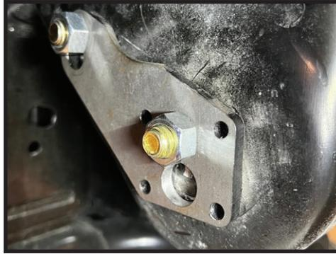
**10.** Using the supplied 20mm hole saw and arbor drill the lower hole that will form the slot.
