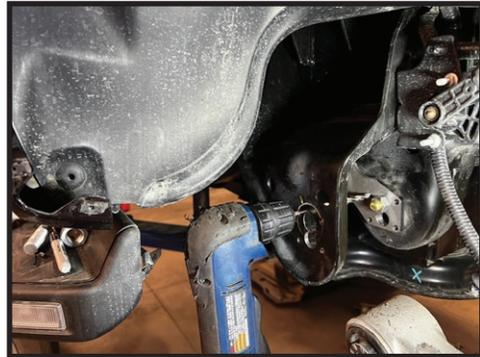
**13.** You may need to remove the splash guard from the front corner of the fender to make room for the drill motor or use a right angle drill.
