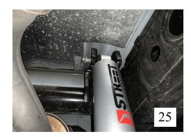
NOTE: Installing the OEM length shocks will not allow for correct travel.
