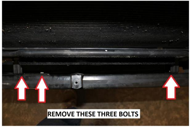
20) Locate the 3 bolts and one nut on each side of the vehicle which secures the front bumper to the chassis. Remove all four fasteners with a 15mm socket and remove the bumper from the vehicle.
