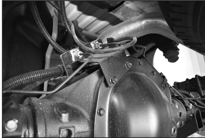
3. Remove the factory shocks, retain all mounting hardware.
