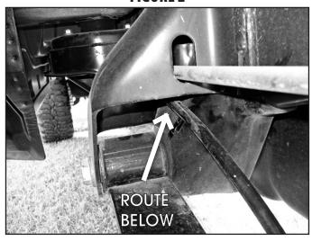
2. Remove the factory rear brake line bracket from the differential cover. (Fig 3)
