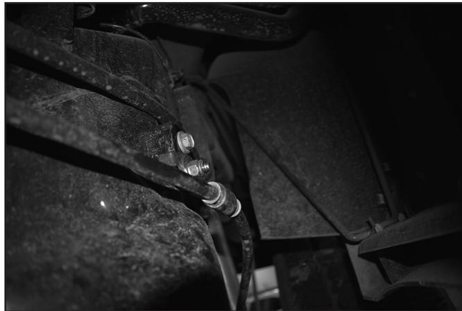
10. Disconnect the rear shocks and lower the axle, retain hardware. On the driver's side it is easiest to access the top hardware by cutting the inner fender well as shown. This trim procedure is not required but greatly aids in removal and installation of the shock. (Fig 5, 6)
