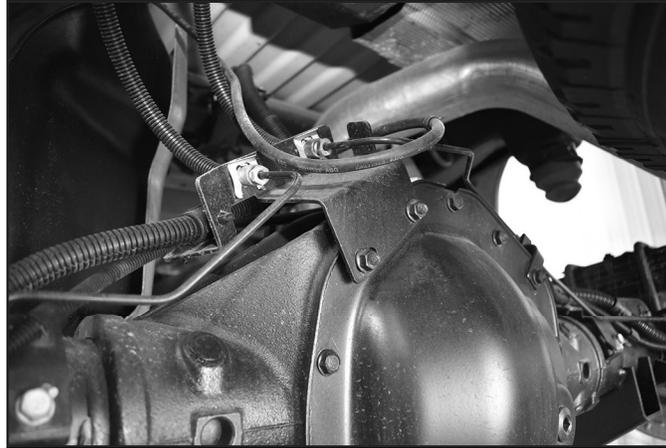
8. If equipped unbolt the power hop damper bracket from the rear axle.
