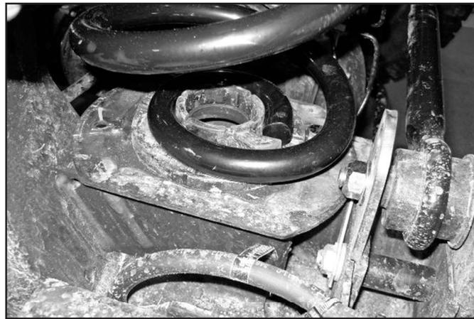
16. Drill out the small hole inside the frame behind the shock mounting hole to 3/8".
