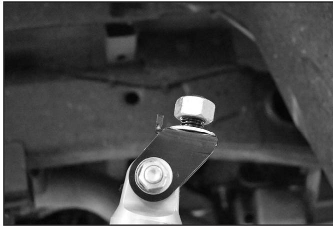
18. Grease bushings and sleeves and install into the sway bar links. Install sway bar links with the new 12mm hardware. (BP 795). Tighten to 45 ft-lbs. (Fig 10)
