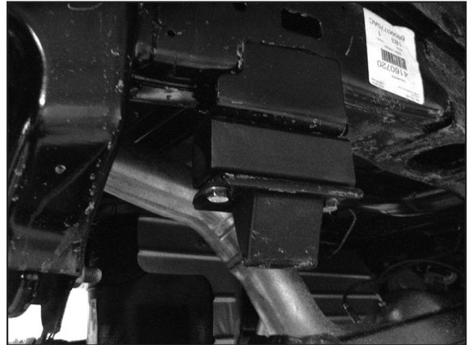
20. Remove the passenger side brake hardline from the passenger side of the differential cover. (Fig 13)
