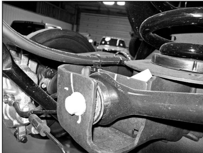
3. Raise the rear of the vehicle and support the frame rails with jack stands.
