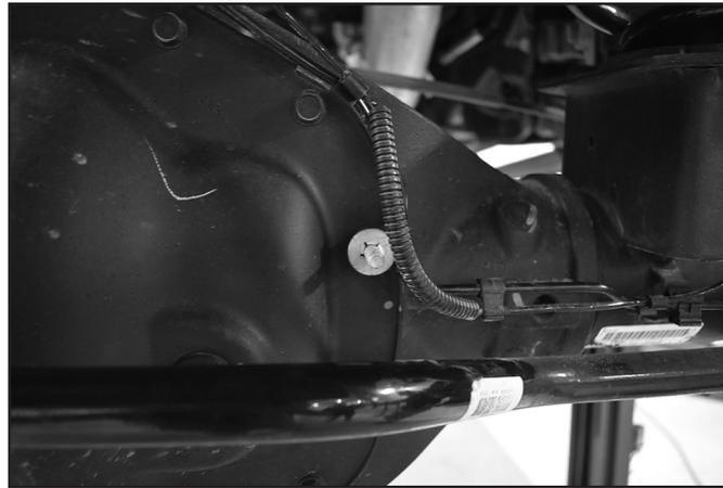
21. Attach the supplied brake line tab to the passenger side hard line with the supplied 5/16" hardware (Bolt Pack 354) and then the tab to the differential cover with the supplied washer and 8mm nut. Torque all hardware to 21 ft-lbs. (Fig 14)
