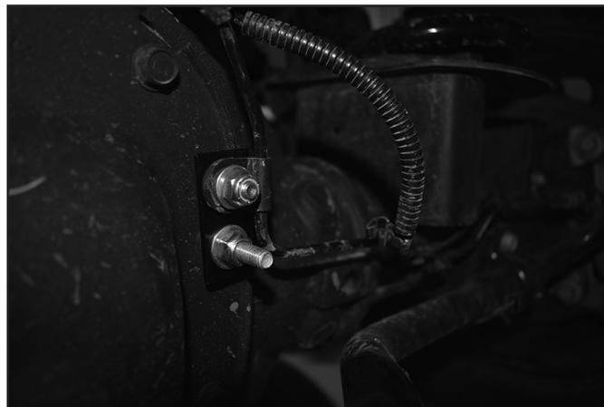
22. Attach the supplied rear brake line bracket to the top of the rear differential cover with factory hardware. Torque to 12 ft-lbs. Use the provided 3/8" hardware (Bolt Pack 356) and fasten the factory brake line bracket to the supplied brake line bracket. Torque hardware to 26 ft-lbs. (Fig 15)
