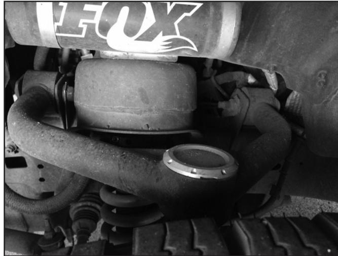
23. **2006-2018 Model year trucks (2019+ skip this step):** Attach the ABS wire to the upper control arm with the included 1/4" hardware with rubber coated clamp. Note the rubber grommet on the ABS wire can be slid on the main cable. Use silicone spray to aid in movement of grommet if necessary. Tighten to 18 ft-lbs.
