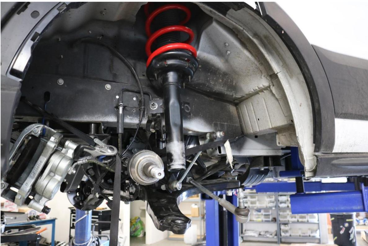
22) With the steering knuckle removed from the vehicle, go ahead and fully remove the lower control arm from the vehicle.
