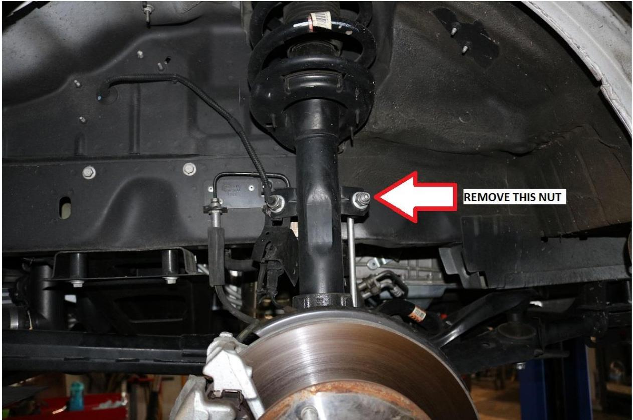
12) Remove the wheel speed sensor wiring from the strut.
