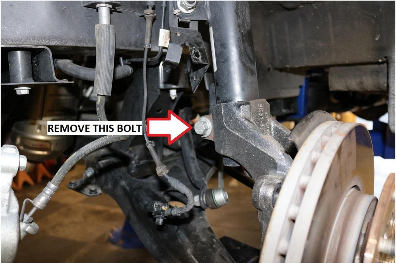
21) Remove the steering knuckle from the strut and set it aside.
