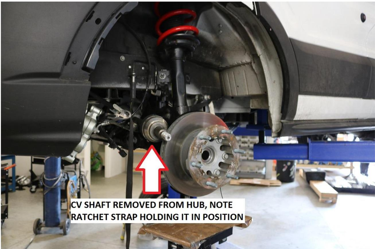
**CV SHAFT REMOVED FROM HUB, NOTE RATCHET STRAP HOLDING IT IN POSITION**
