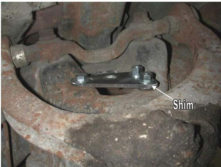
4. Remove the factory upper shock mount. The front of it is held in with two rivets that must be ground down and pushed out. In its place install the upper air spring mounting plate & shim. The shim will go under the front side of the plate and is secured with two 3/8" x 1 1/2" bolts, flat washers, nuts and lock washers. The rear side of the plate will be secured with one 3/8" x 1 1/4" bolt flat washer and lock washer.
