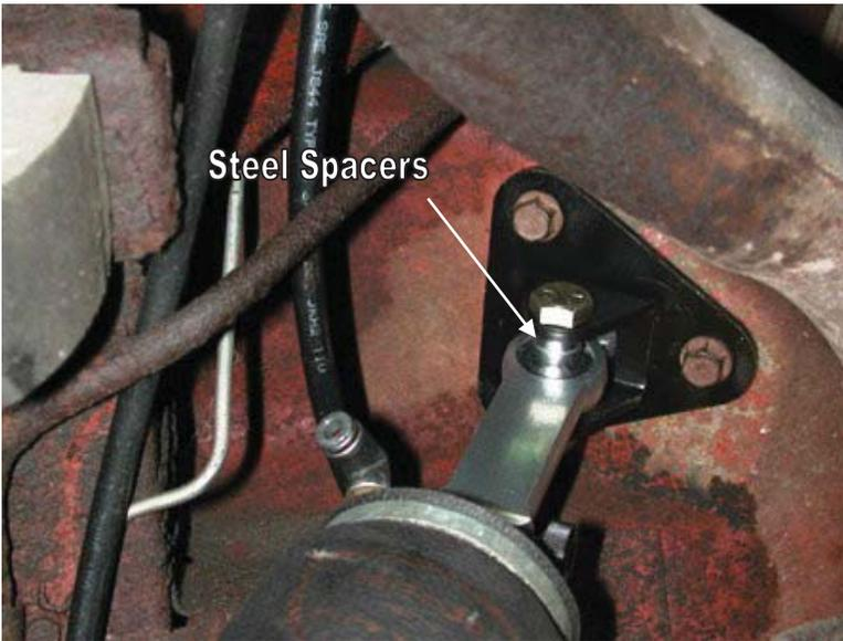
9. Bolt the plate to the factory shock mount holes using the factory bolts. The ShockWave must be bolted to the car with the upper mounting bolt running front to rear.
