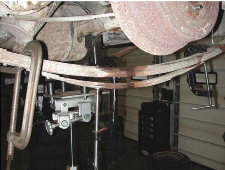
3. To get maximum drop, the two lower leaf springs must be removed from the pack. Raise the U-bolts clamping the axle to the leaf spring pack. Raise the axle out of the way with a floor jack. Secure it with two jack stands.
