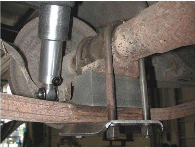
7. Hang the U-bolts over the axle. Position the U-bolt plate under the leaf springs so that the smaller hole in the plate aligns with the Allen bolt and nut. Secure the assembly with the four 5/8" nuts and lock washers supplied.
