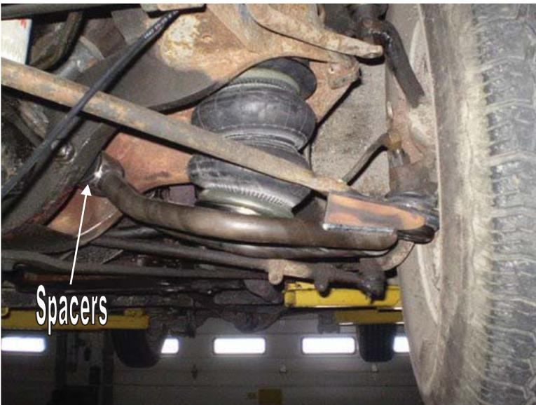
9. Bolt the lower StongArm to the frame using the 3/4" x 8" bolt and the two spacers supplied. Install the 1" spacer to the front side of the bushing and the 1 7/16" spacer to the rear. A large washer will go between the bushing and the spacers.
