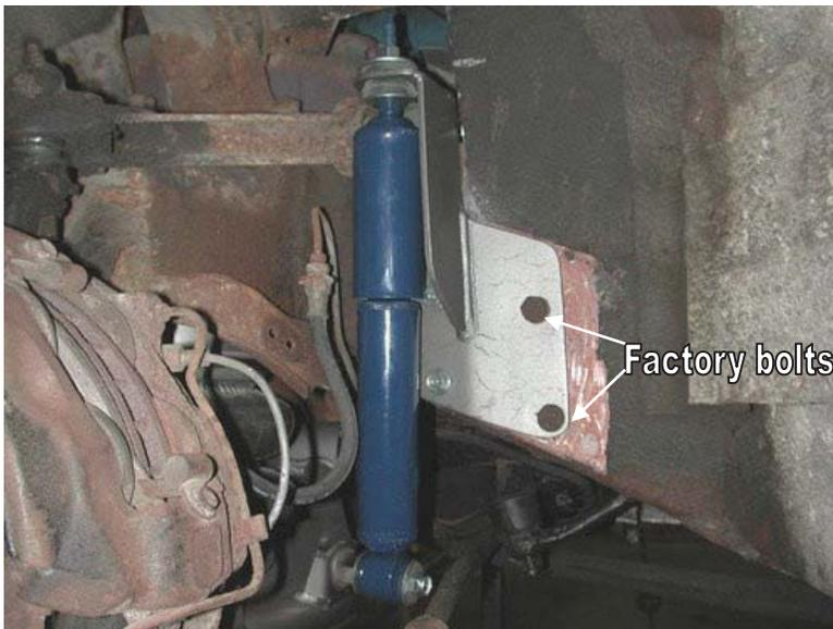
4. Bolt the top of the shock to the upper mount using the bushings and hardware supplied.
