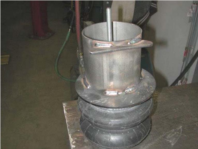
6. Thread the 7/16" x 6 3/4" stud into the nut in the bottom of the bracket.
