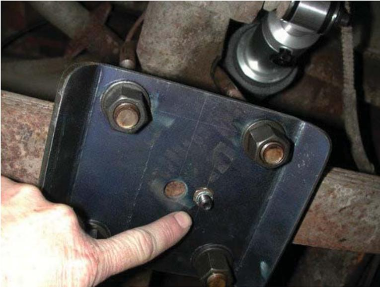
5. Secure the pack with a 3/8" x 2" Allen bolt and Nylok nut. The bolt needs to be dropped in from the top of the pack. Reinstall the straps then remove the clamps.
