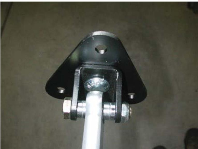
8. Insert a 1/2" ID shock bearing spacer in each side of the shock bearing. The small OD will go into the bearing. Bolt the Shockwave to the eye to stud adapter using the 1/2" x 2 1/4" bolt and Nylok nut.
