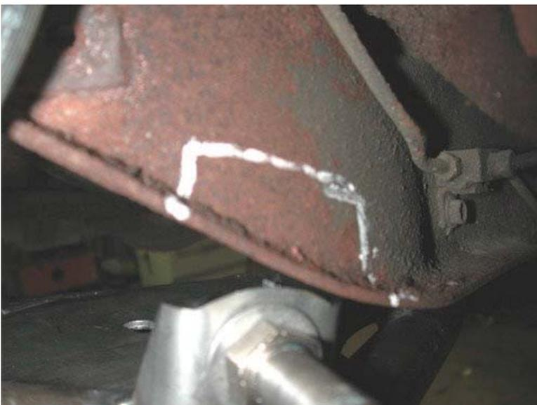
12. Raise the lower arm with a jack. Mark the frame where the lower shock tab contacts it. This must be cut out to allow clearance. Grind all edges smooth when finished.
