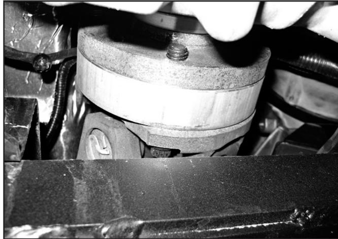
16. Reinstall the transmission mount with factory hardware.
