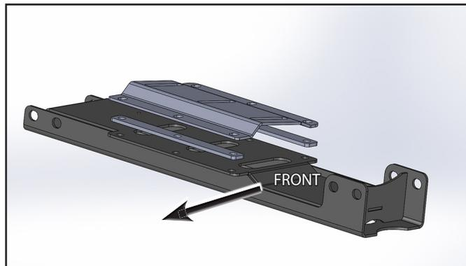
18. Install new crossmember with factory bolts. If this installation is combined with a BDS 4-link kit the nuts will not be put on at this time, and will need to be installed with the 4-link brackets. Otherwise tighten to 150 ft-lbs.
