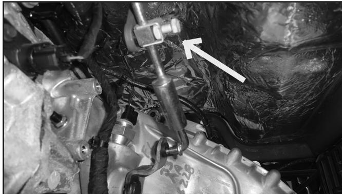
22. When adjusting the shift linkage, it is best to keep the shift linkage in 2wd. Loosen the bolt attaching the rod to the shifter lever going into the cab of the truck (Fig. 9B).
