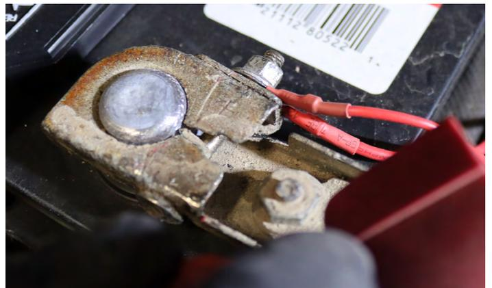
After connecting the wire harness to the battery, guide it towards the driver's side of the headlight location.
