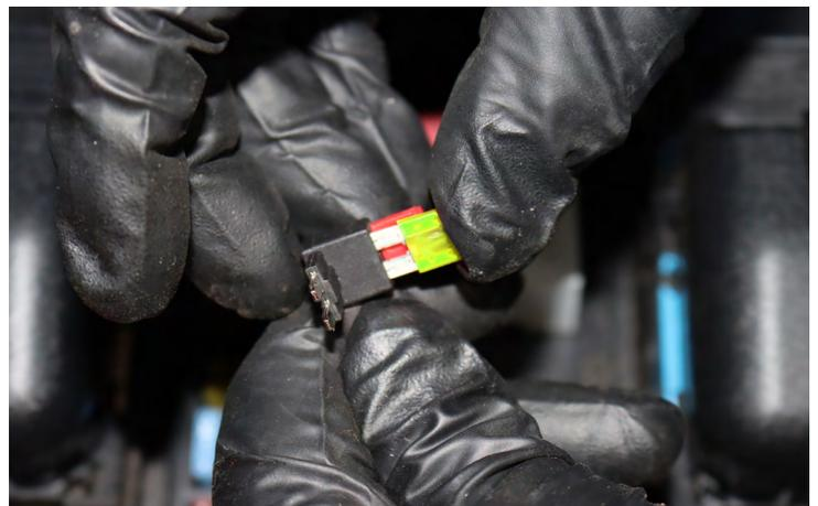
Once the fuse box cover is closed, route the DRL harness wire towards the driver side of the headlight location.
