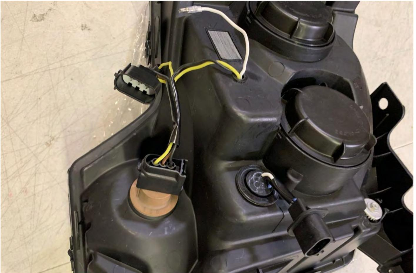
After transferring the sockets to the new ALPHAREX headlights, the assembly should now resemble this configuration.
