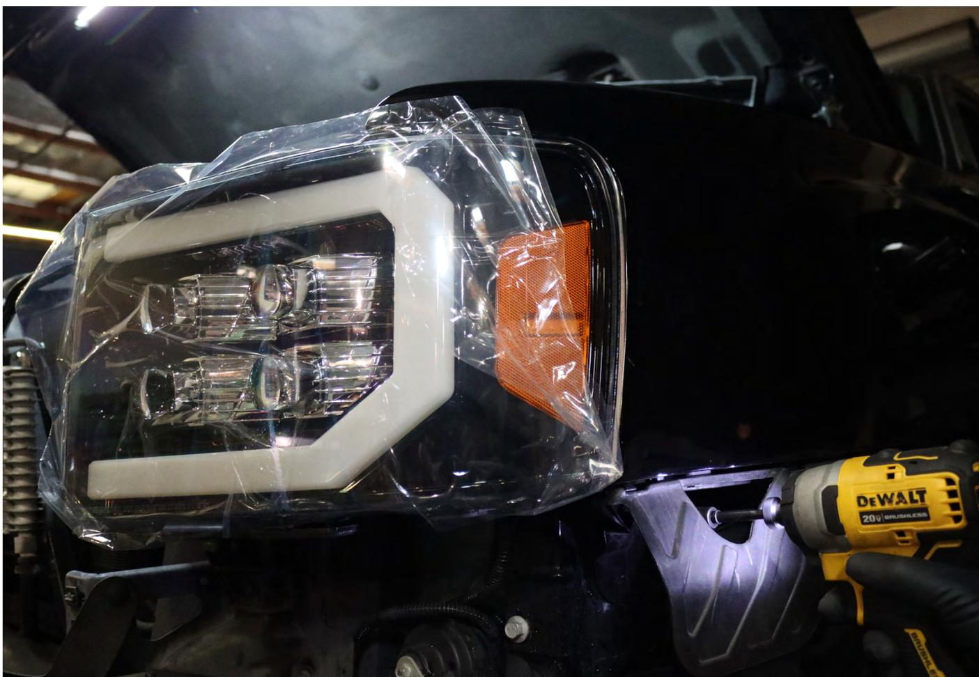
To complete the installation, reverse the process of removing the bumper and grille. Follow the previous steps in reverse order for reassembly.
