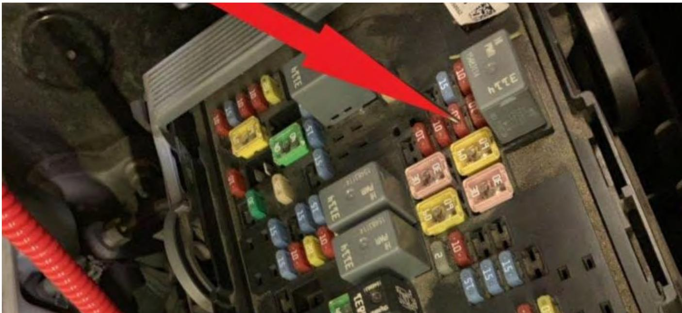
After tapping into the fuse, proceed to route the DRL harness wire to the other side of the headlights.
