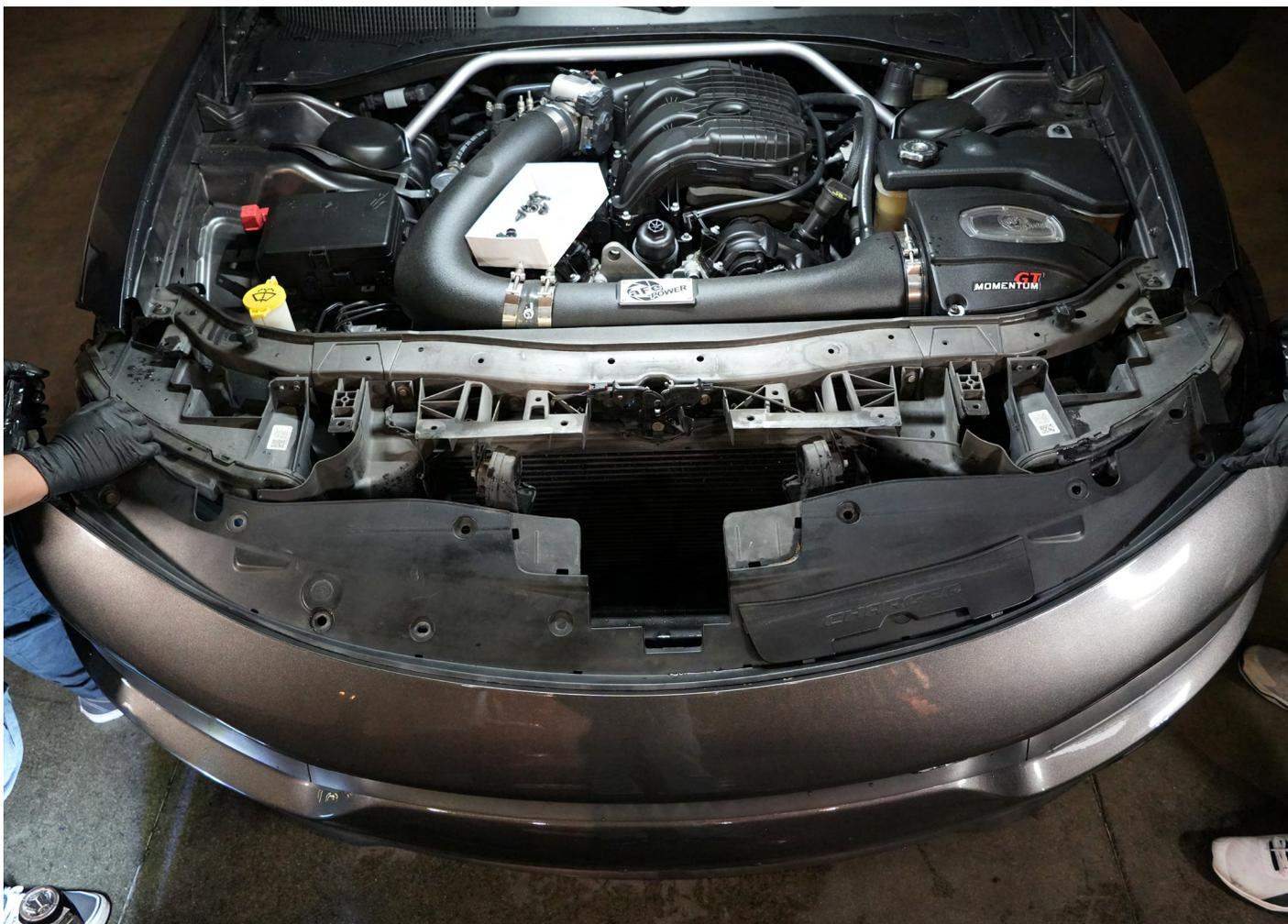
Disconnect the fog light connectors and side marker connectors, then proceed to remove the front bumper entirely. Set it aside for later reinstallation.
