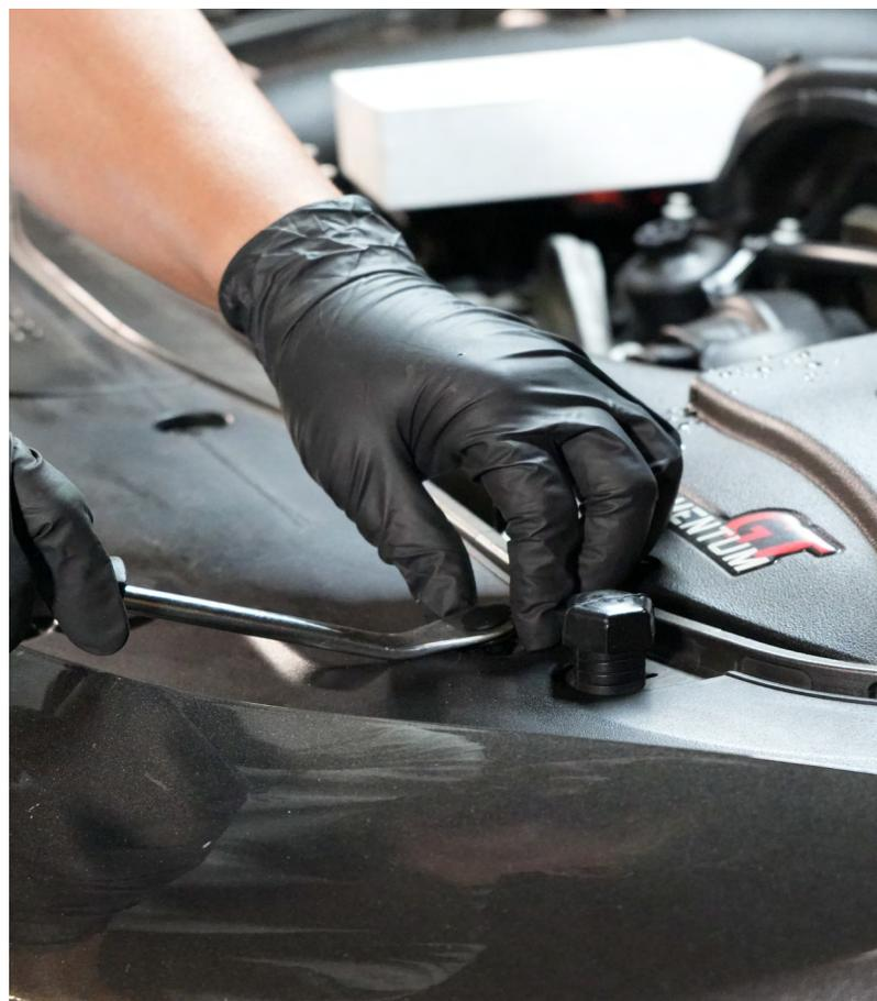
Remove the two 10mm bolts, located individually on either side of the upper bumper corner.
