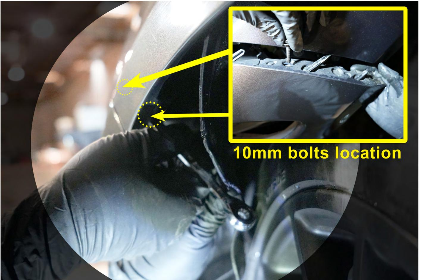
Repeat the identical steps on the opposite side of the wheel fender. Open the fender liner widely and remove the two 10mm bolts securing the front bumper.
