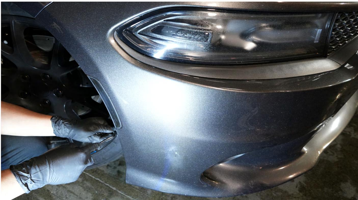
Take out the eight 7mm bolts located underneath the front bumper.
