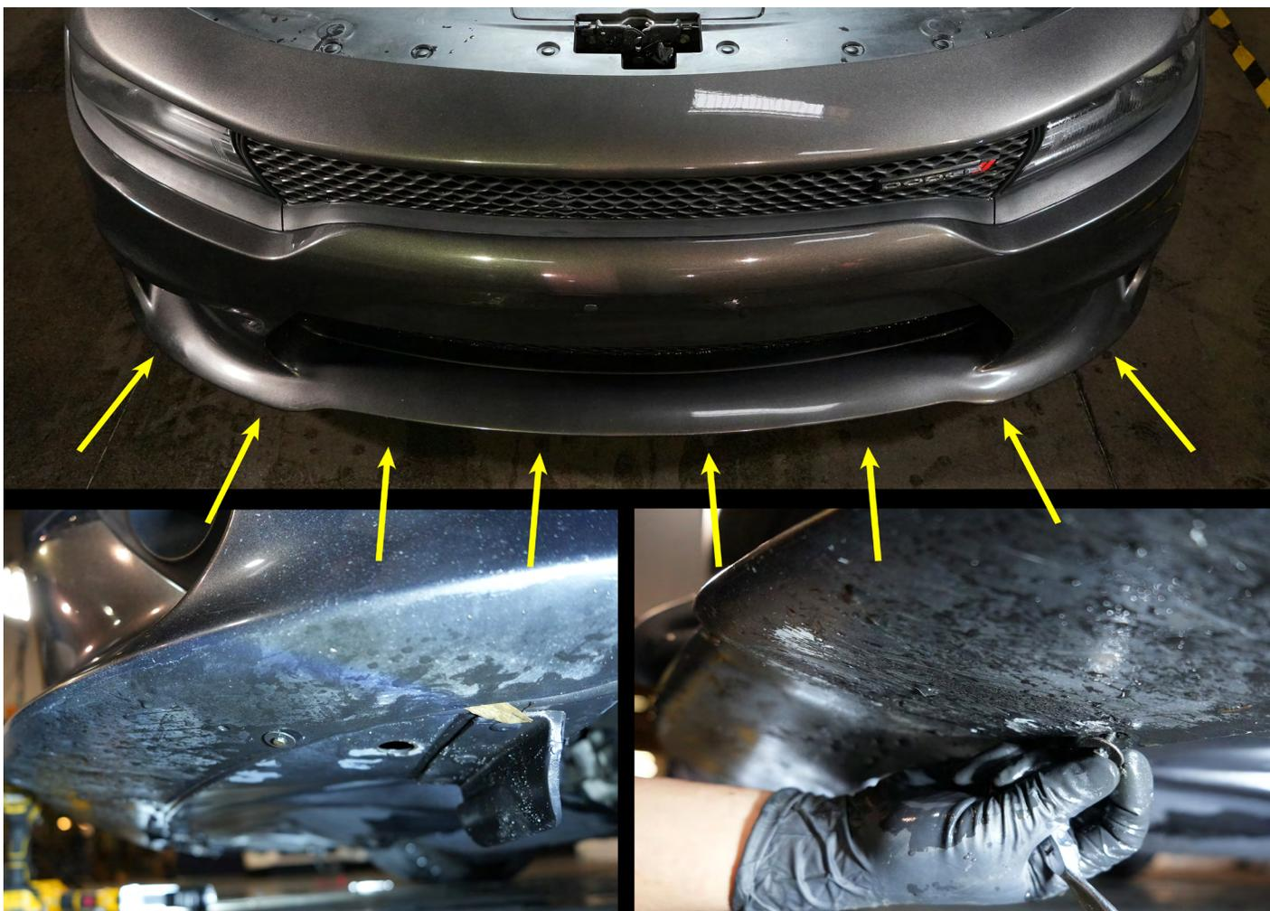
Gently detach the front bumper by pulling outward from each side, disengaging it from the mounting clips.
