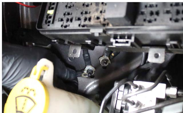
To initiate, open the fuse box and tap the red wire into the fuse F39 (10A).
