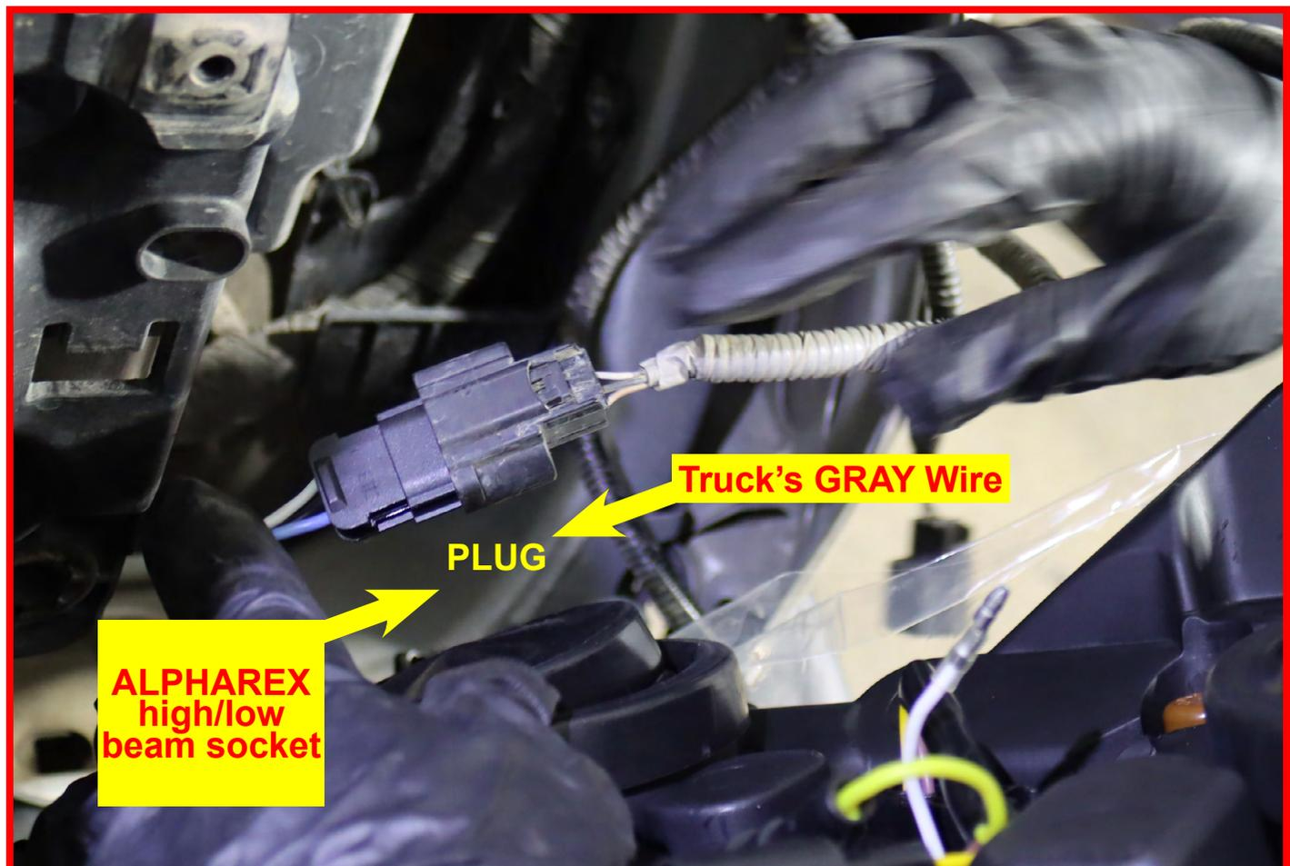
Connect the turn signal and parking light wires into the new ALPHAREX headlight.
