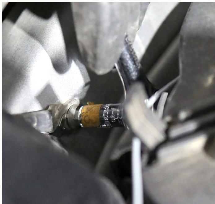
Guide the DRL wires to both sides of the headlights.
