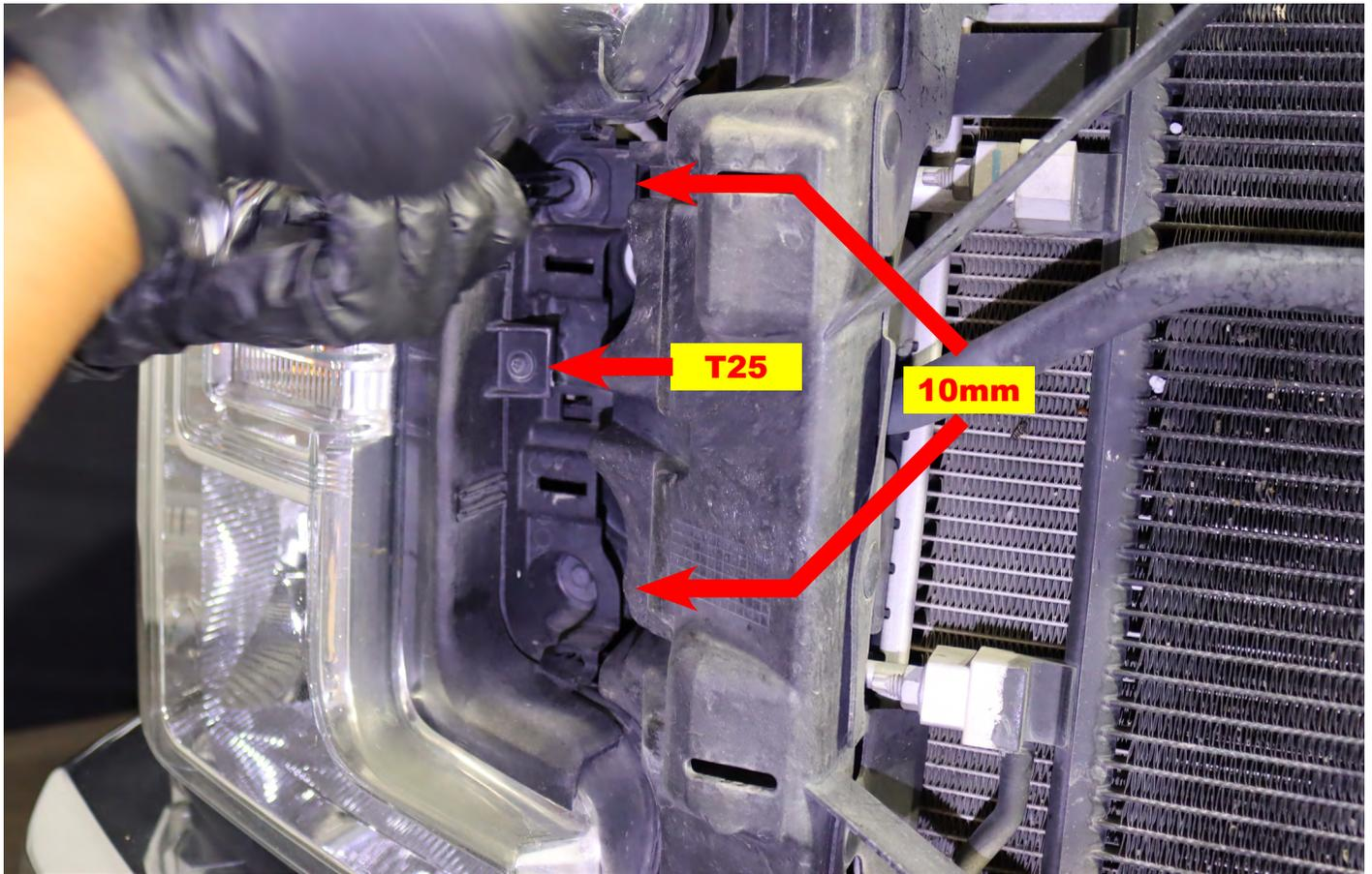
Utilize an extension to assist in removing the 10mm bolt from the side of the headlight, located inside the front fender and bumper mounts. Repeat these steps for the other side of the headlight.
