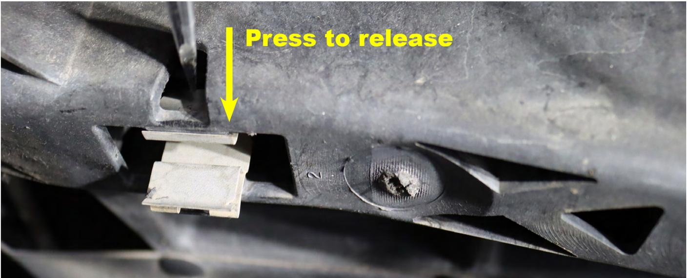
Subsequently, gently pull the grille outward towards you to disengage it from all the mounting points and remove the front grille. If your truck is equipped with a Front View Camera Washer, ensure to unplug the nozzle's tube and the wiring before removing the grille.
