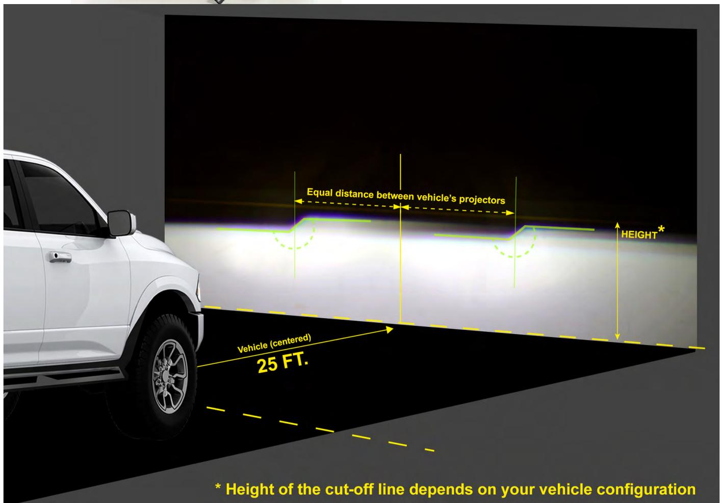
**\* Height of the cut-off line depends on your vehicle configuration**
