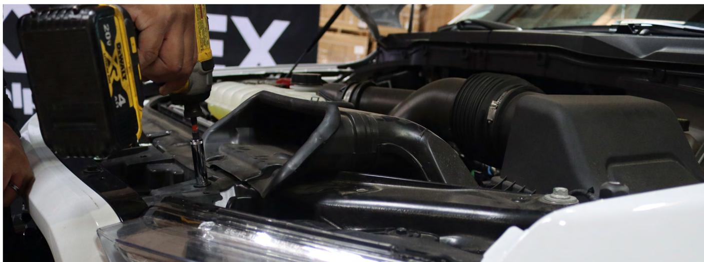
Release the two plastic tension clips and gently pull the grille assembly outward to remove it. Set the assembly aside for future reinstallation.
