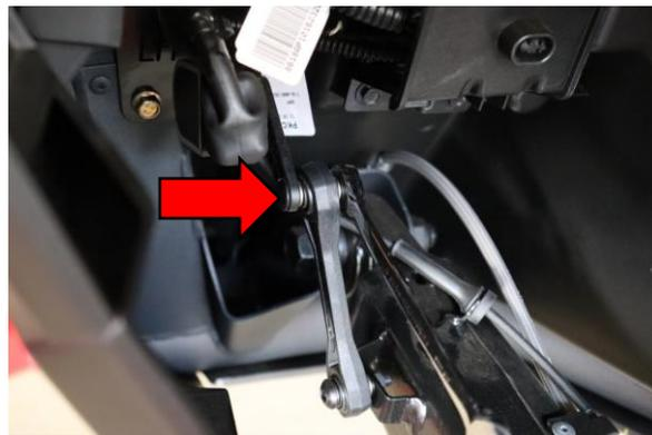
Step 2. Remove 10mm nut and T30 bolt from ride height sensor arm at front of lower trailing arm.
