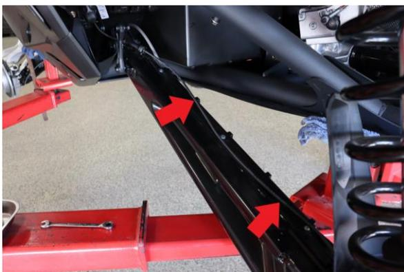
Step 3. Remove lower shock wire harness from clips along lower trailing arm.
