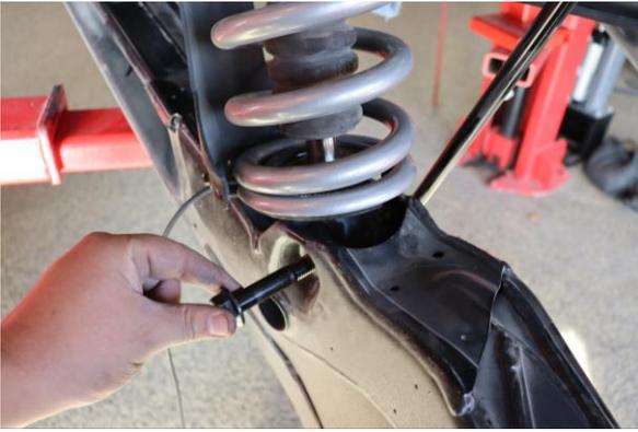
Step 7. Remove 21mm lower shock nut and bolt. (This bolt from the manufacturer has a yellow Loctite that may require a large breaker bar to remove).
