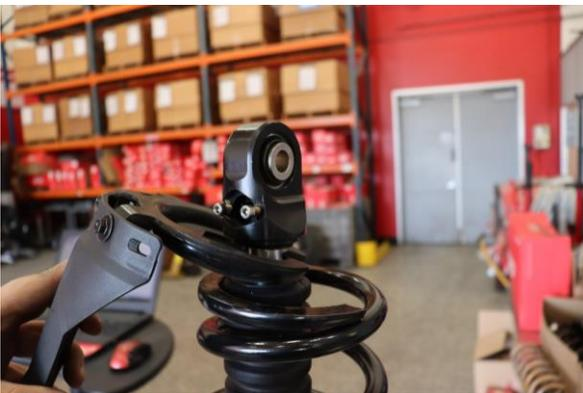
Step 11. Use a spring compressor to compress spring assembly. Remove lower spring retainer.
