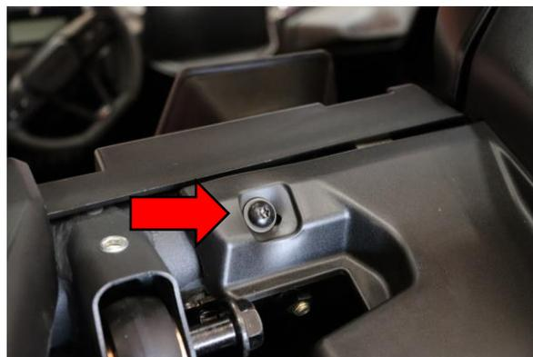
Step 6. Remove T30 screw from rear deck panel near upper shock mount.
