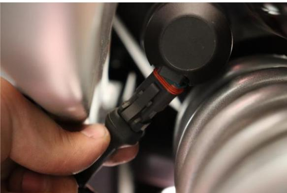
Step 27. Install the upper shock wire harness at the shock assembly.
