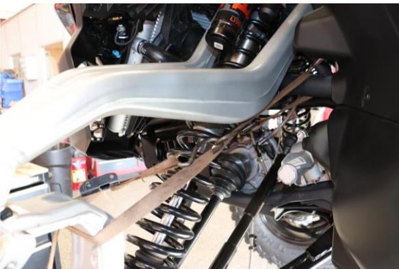
Step 5. Secure the spindle to the frame to prevent damage to the axle CV joints.
