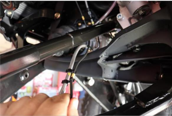
Step 3. Remove lower shock wiring harness from retaining clips along the brake line.
