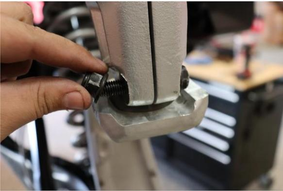
Step 25. Lower the upper control arm onto the upper ball joint and install retaining bolt. Use two 15mm sockets tighten to manufacturer specification.
