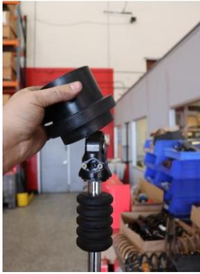
Step 13. Remove spring slider.
