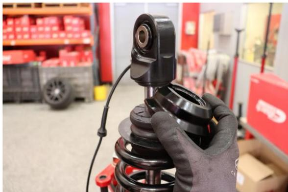
Step 12. Remove the spring retainer.
