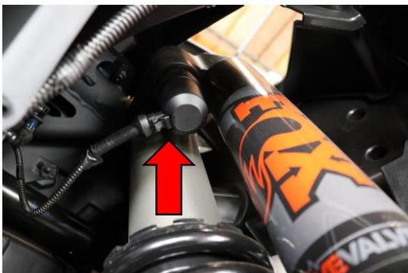
Step 5. Disconnect upper shock wire harness at shock assembly.
