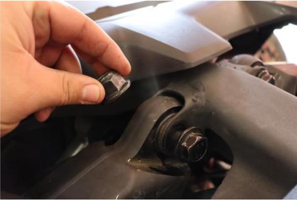
Step 24. Install upper shock mount nut and tighten to manufacturer specification using 21mm socket and wrench.
