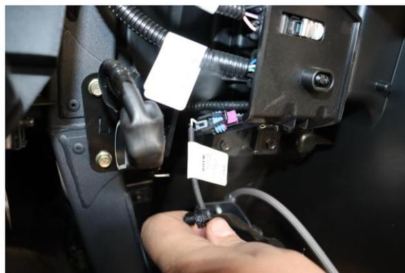
Step 4. Disconnect lower shock wire harness at front of trailing arm.
