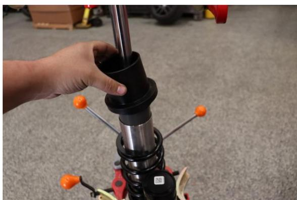
Step 14. Remove spring slider.
