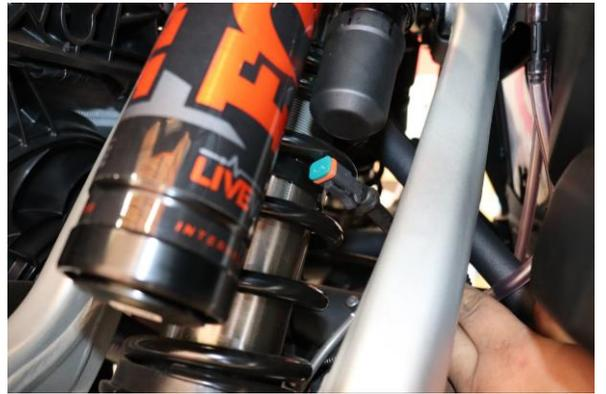
Step 4. Disconnect upper shock wiring harness at shock body.
