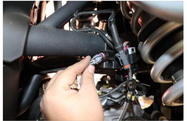
Step 26. Route the lower shock wire harness along brake line clips and connect at frame.
