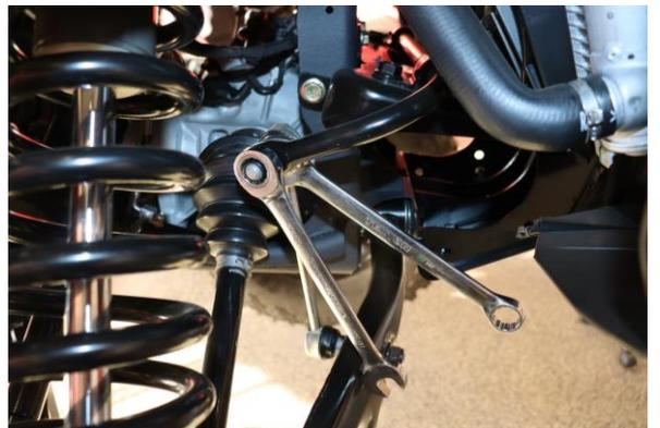
Step 6. Use 19mm wrench and 18mm socket to remove left and right sway bar end links.
