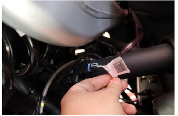
Step 2. Remove lower shock electrical connector at frame.
