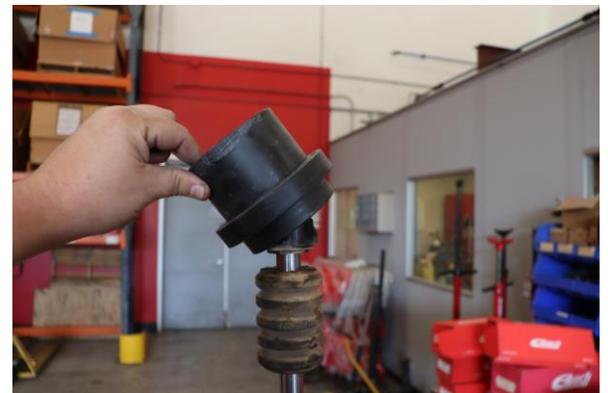
Step 18. Reinstall OE spring slider.
