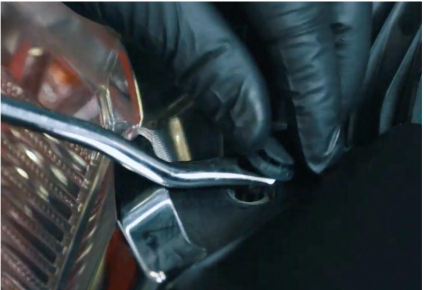
Remove the grille from the truck and set it aside to be reinstalled.
