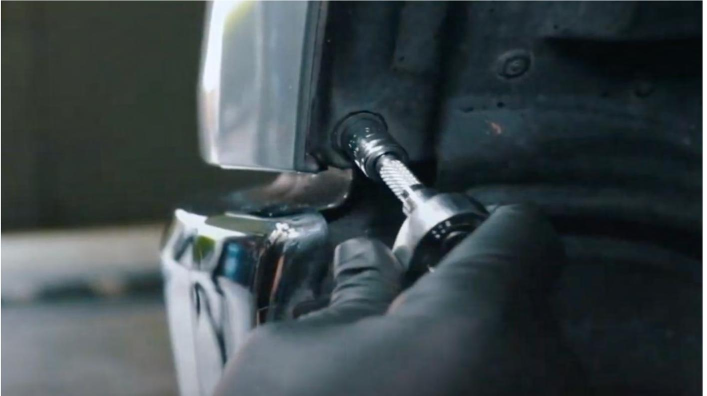
Remove the clip located on the inside of the trim piece.
