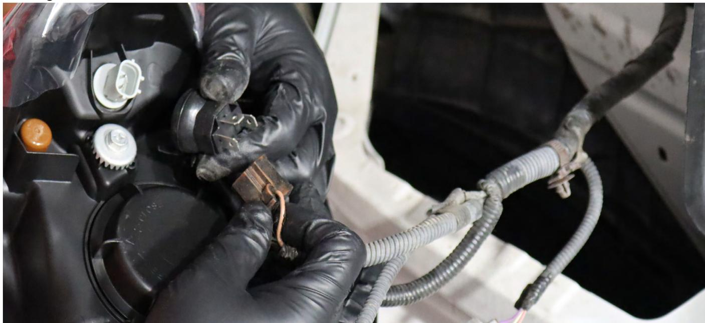
Attach the harness to the daytime running light connection on the back of the headlight.
