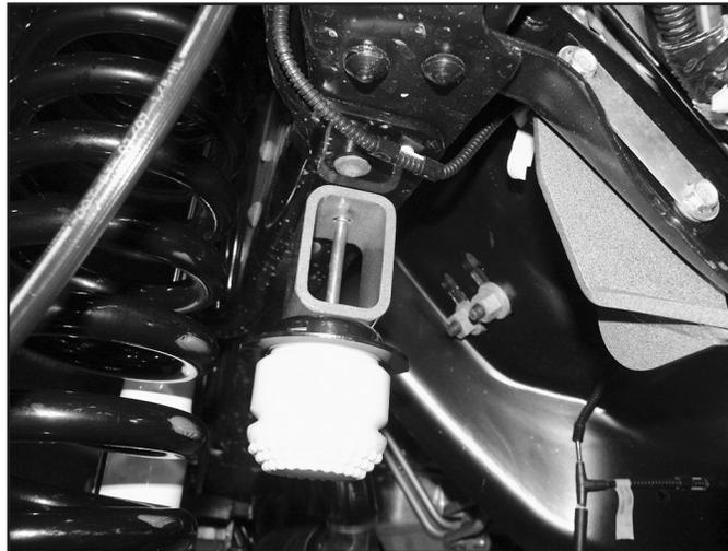
25. Loosen the four radius arm-to-axle mounting bolts but do not remove. Once again, ensure that the front axle is well supported.
