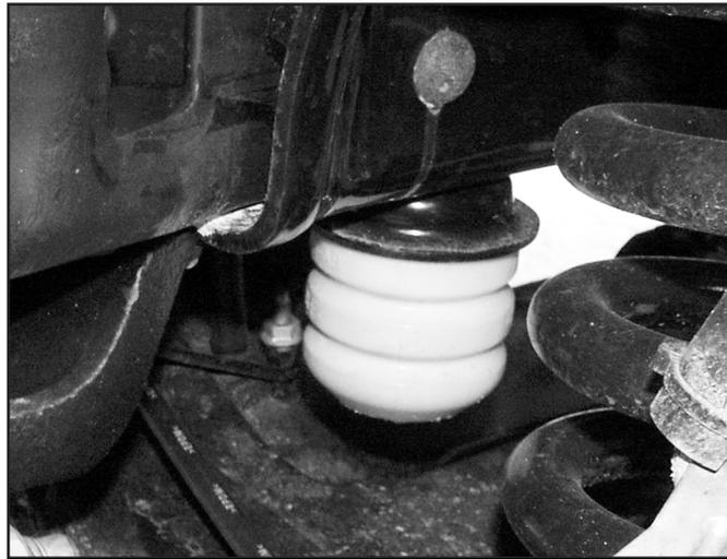
23. Position the cup on the provided bump stop extension. The alignment tab on the bump stop cup will fit in the second hole in the extension.
