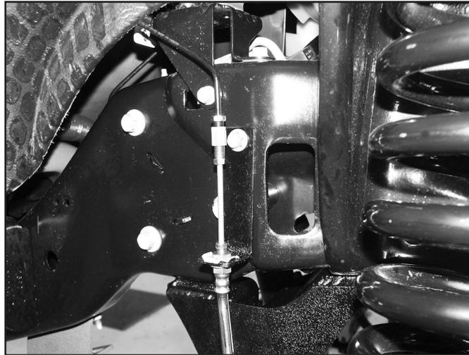
53. Properly bleed the brake system of air and top off the brake fluid reservoir with the proper type of fluid (see owners manual).
