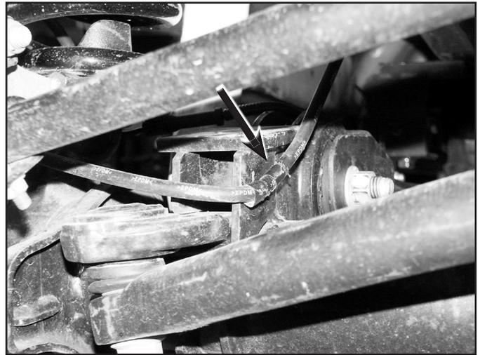
8. Disconnect the sway bar end links from the sway bar. Retain hardware.
