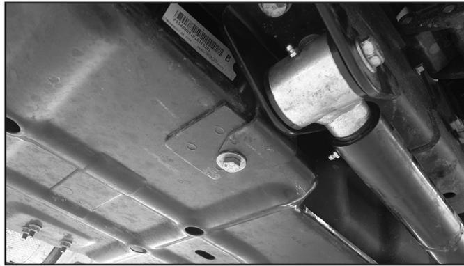
21. Mark the hole location for the skid plate support bracket on the bottom of the fuel tank skid plate.
