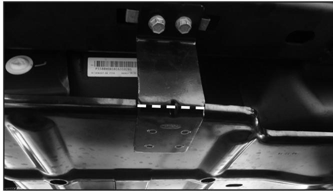
11. Remove the two bolts that are attached to the upper part of the fuel tank skid plate support that was just cut. Remove the two J-nuts from the frame rail.
