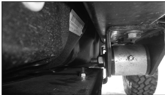
24. Lightly grease the slider end of the traction bar by hand to work grease into the O-ring seals. The traction bar slider end may need to be pulled out a bit and rotated so the grease can fully be worked into the O-rings.
