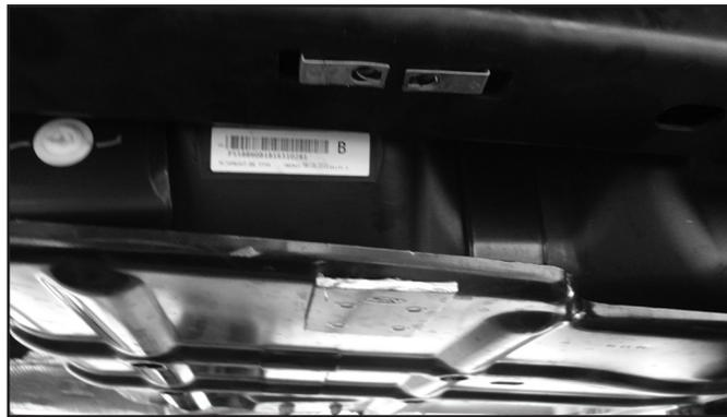
12. Starting on the driver's side, loosely attach the frame bracket (02876) with a 9/16" x 4-1/2" bolt from Bolt Pack 984 and a 9/16" nut and two 9/16" SAE washers from Bolt Pack 964 to the Traction Bar Slider End (02869). Make sure the frame bracket is installed such that the single hole is towards the front of the vehicle and the two slots are towards the rear of the vehicle.
