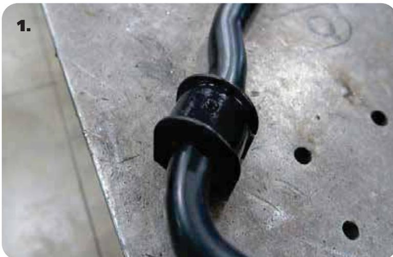
1. Apply lithium grease to the poly bushing. Install the bushing over the sway bar.
