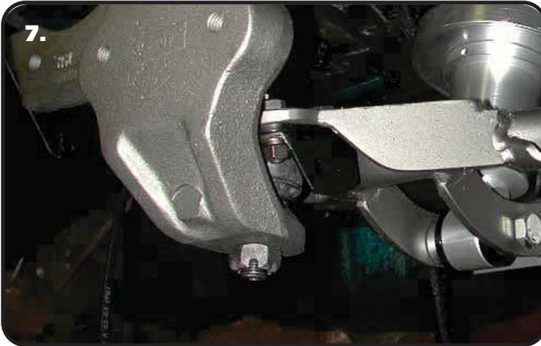
7. Attach the Spindle to the control arms.
