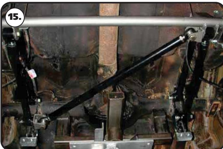
**15.** Swing the axle bracket up to the axle. These brackets must be centered and aligned with the crossmember mounts before welding. The brackets should be 31 5/8" apart on the outside measurement. Then just center it between the axle flanges. You can use a large hose clamp to hold these in place temporarily.
