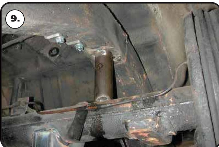
9. Pinion angle must be set at ride height. At ride height there should be 4 1/2" between the axle and frame. One trick to help maintain these setting while welding in the axle bracket is to tack weld a 4 1/2" long spacer between the axle and frame. **Refer to Page 8 for pinion angle setting.** After setting the pinion angle, make sure the axle is centered. This can be done by measuring from the axle flange in to the frame rail.
