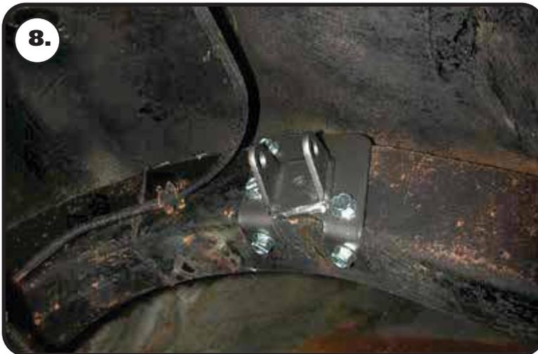
8. Use a clamp to hold the bracket against the inside of the frame and drill the holes with a 5/16" bit. Thread a 3/8" x 1" self-tapping bolt into the frame after drilling each hole.
