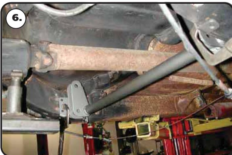
6. Use a couple clamps to secure the crossmember between the frame rails. Slide it forward to the edge of the body mounts. Drill the holes with a 5/16" bit and thread the 3/8" x 1" self-tapping bolts in one at a time.
