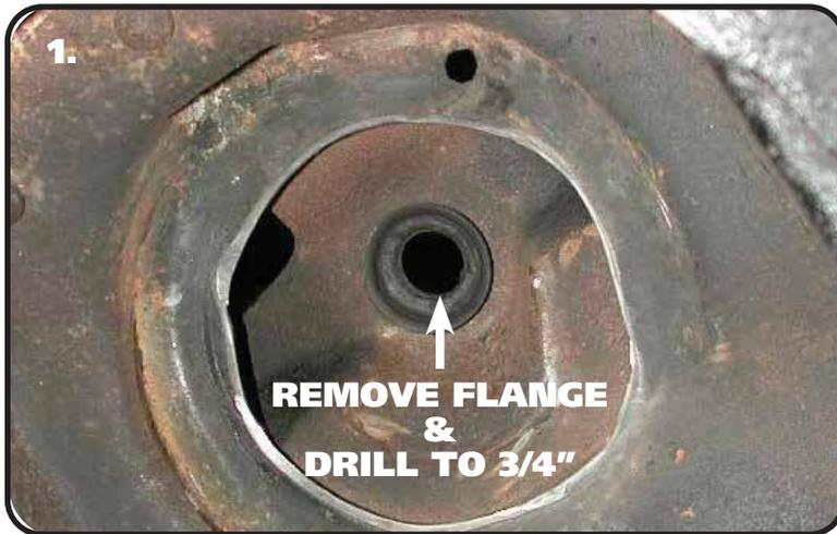
1. Remove the OEM bushing flange by prying it out of the frame hole. After removing the flange, drill the OEM shock hole out to 3/4". This can be done with a Unibit.
