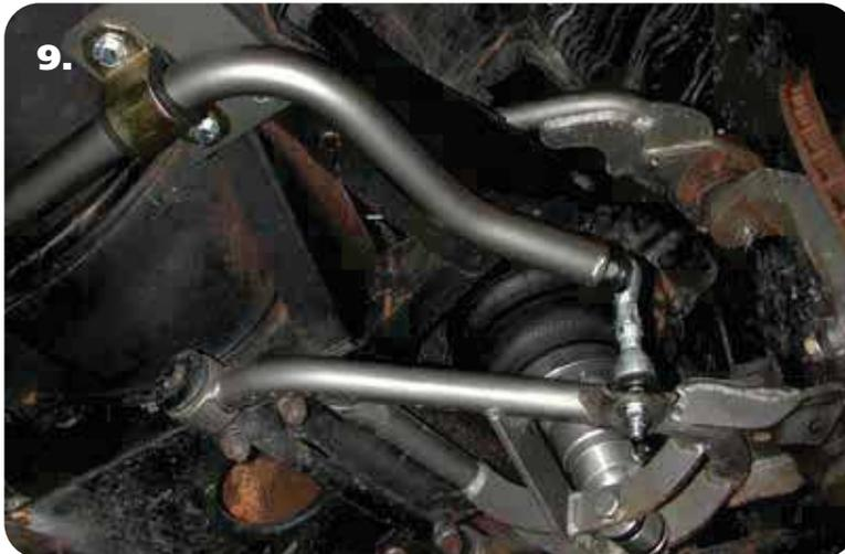
9. Bolt the 90 degree end of the PosiLink to the sway bar. A 3/8" flat washer and 10mm lock washer must be installed between the PosiLink and the bar.
