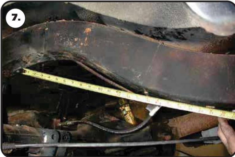
7. The location of the upper Shockwave mount is determined by measuring from the front edge of the bracket to rear edge of the large hole in the bottom of the frame. The location of the large locating hole varies between the 1 piece frame and 2 piece frame. Use the correct measurement from below to locate your shock mount.
