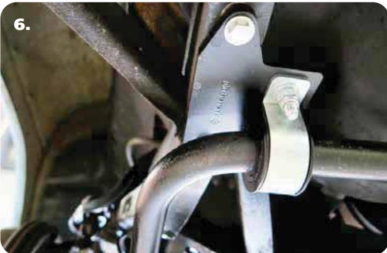
6. With the bushings and straps installed on the sway bar, put the swaybar in position on the 3/8" bolts. Attach it using 3/8" flat washers and 3/8" nylok nuts. Do **NOT** completely tighten the hardware. It will be left partially loose until the PosiLinks are installed.
