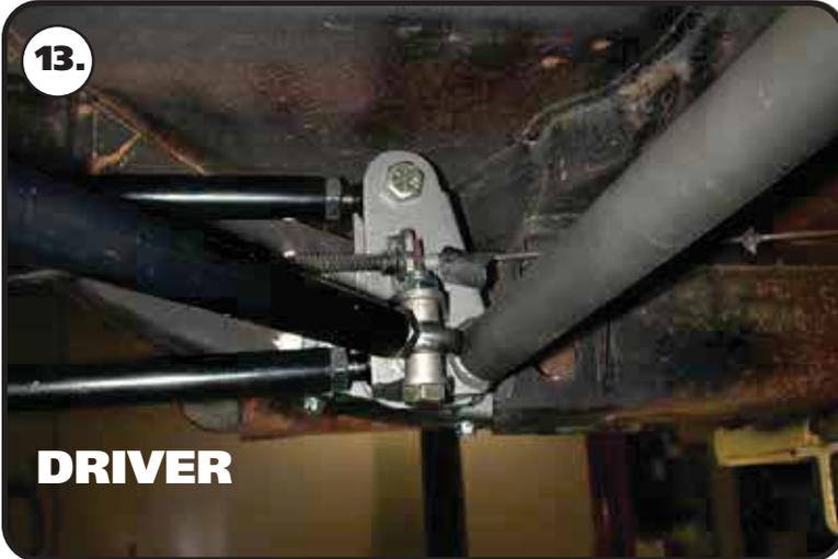
**13.** Insert the R-Joint spacers into the R-joint with the small OD inserted into the R-Joint center pivot. Bolt the diagonal link into the mount on the cross member using a 5/8" x 2 3/4" bolt and nylok. It should measure 30 1/4" center to center. Tighten the bolts/nuts enough to eliminate any gaps.
