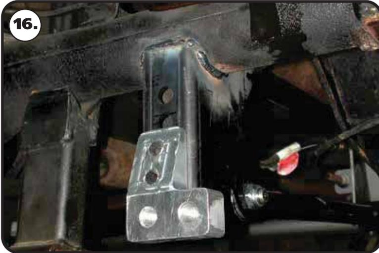
**16.** Bolt the lower Shockwave mount to the axle bracket using (2) 1/2"-20" x 3/4" hex head bolts. The mount offsets the lower shock stud to the outside of the car. Attach the mount to the **2 BOTTOM** holes of the axle mount. Torque the bolts to 75 ft-lbs.
