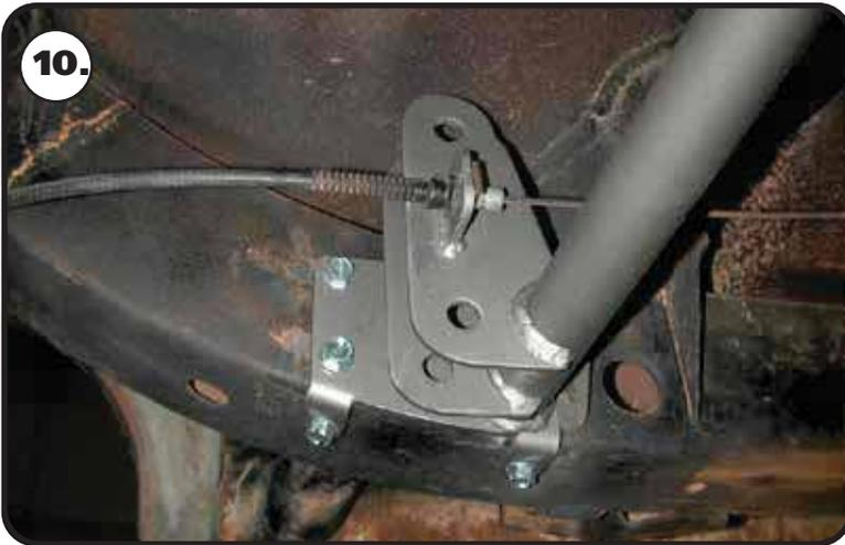
10. Reattach the emergency brake cables to the mounts built into the front cross member.
