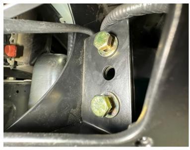
32. Adjust the light alignment as necessary, then use a 9/16" to toque the hardware to 25lb/ft.
