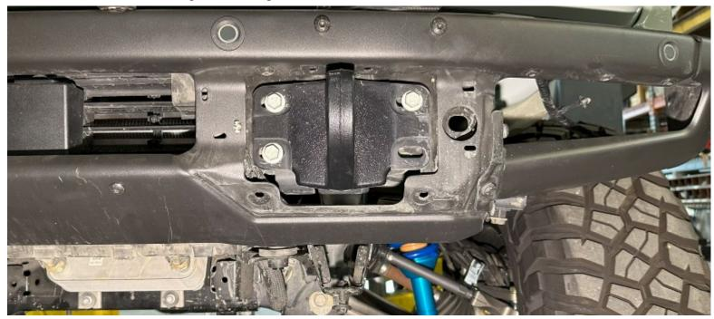
4. 15MM Socket — Remove the 6 bolts retaining the factory bumper. And remove the bumper.
