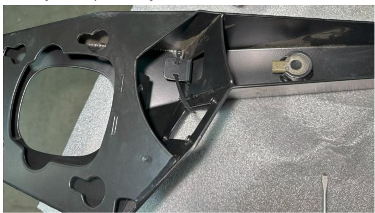
27. Slide the wing onto the bolts and tighten using a stubby 3/4" wrench. Torque to 64lb/ft where possible.
