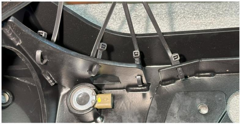
17. Install the parking sensor harness and provided light harness (for the Baja Designs S2 and XL80) into the center channel ensuring all connections are internally routed through the designed passages AND have sufficient slack to reach all sensors and lights. Once confirmed, secure zip ties and cut off excess. (more pictures on next page)
