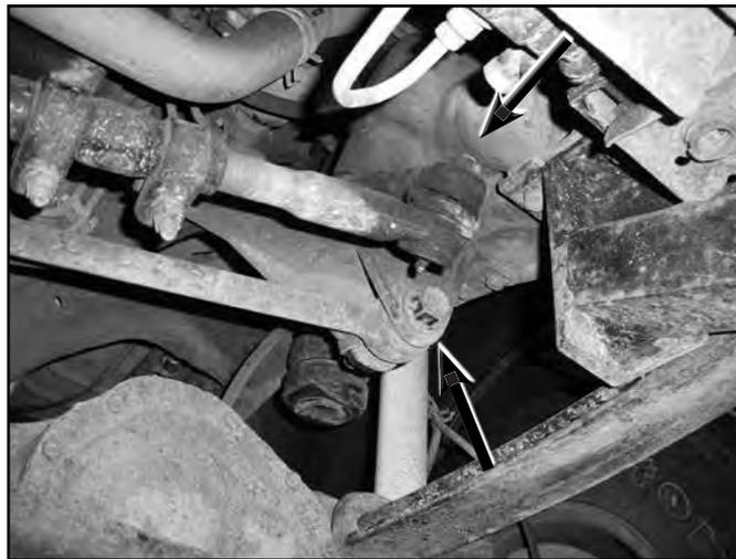
7. Remove the front shocks from the axle and frame mounts. Save hardware and discard shocks.
