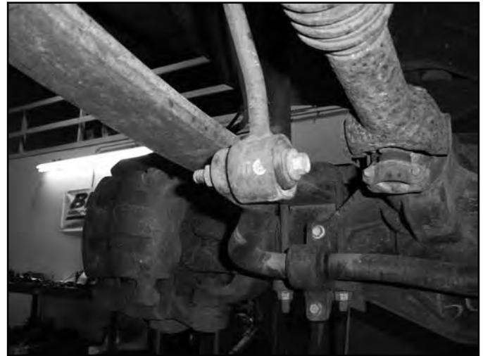
10. Disconnect the front drive shaft from the front axle. Save u-joint straps and bolts.
