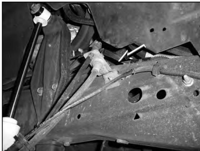
9. Disconnect the front sway bar links from the sway bar and frame (Fig 3A,B). Remove the links from the vehicle and discard. Save hardware. Note: Some early model vehicles had sway bar link mounts below the frame. The newer style frame mount is shown in Fig 3A
