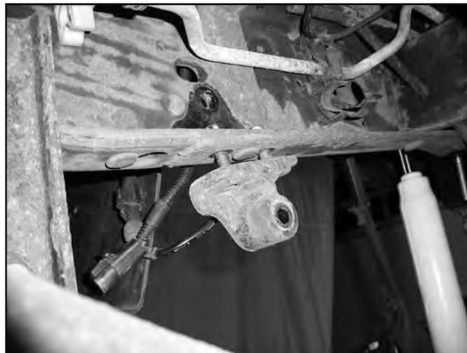
25. Locate the original brake line bracket mounting hole on the frame. Measure down 3" and forward 2" from the original mounting hole and drill a new bracket mounting hole. Check the inside of the frame for wires/hoses before drilling. Carefully reform the brake lines to reposition the mount bracket. Bend the alignment tab on the bracket flat and reattach the bracket to the frame with the original bolt. Torque bolt to 15 ft-lbs.
