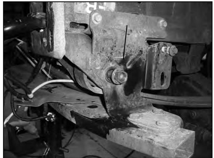
12. With all of the leaf spring bolts loose, support the passenger's side of the front axle with a jack. Remove the passenger's side spring u-bolts. Lower the axle away from the spring. Remove the spring bolts and remove the spring from the vehicle. Save the leaf spring bolts and discard the u-bolts.
