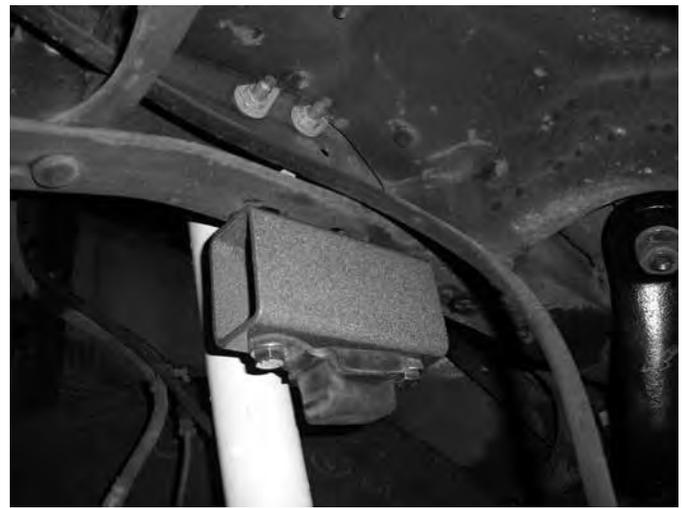
21. Install the new provided shocks to the factory axle/frame mounts with the original hardware. The body end of the shock mounts to the axle. Torque the upper and lower shock mount hardware to 70 ft-lbs
