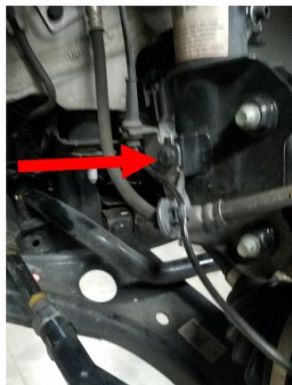
With an adjustable jack under the lower control arm, remove the strut to knuckle fasteners. Retain factory hardware.
