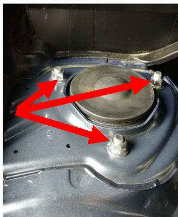
Locate the ReadyLIFT front strut extension. Align the bottom of the R logo with the mount for the knuckle. Install to the top of the strut using the **factory hardware**. Torque to 30 ft-lbs.
