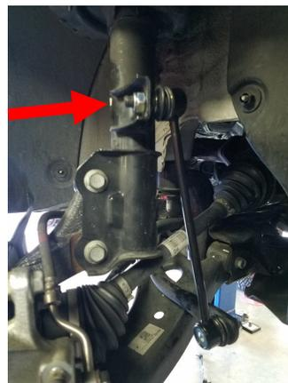
Remove the **brake line bracket and ABS wire** at the strut body. Let hang out of the way. Retain factory hardware.
