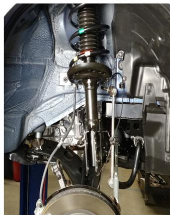
Raise the knuckle up and install into the strut body. Install the **bolt into the upper hole** and the remaining **bolt into the lower**. Torque to 90ft-lbs.
