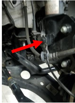
Attach the sway bar end link bracket to the strut assembly. Use provided hardware torque to 65ft-lbs.
