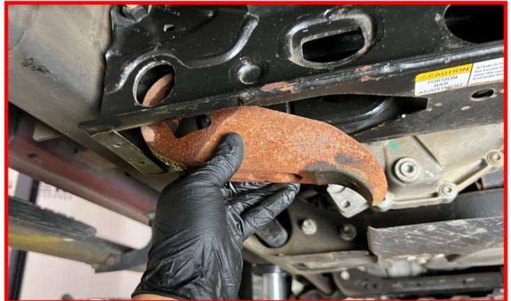
Install the ReadyLIFT keyway into the cross member while sliding the torsion bar into place. The tang of the keyway will be clocked slightly lower than the factory key. This accounts for the lift. Do not load the cross pin or bolt adjuster at this time. This will be done as one of the last steps in the front install.
