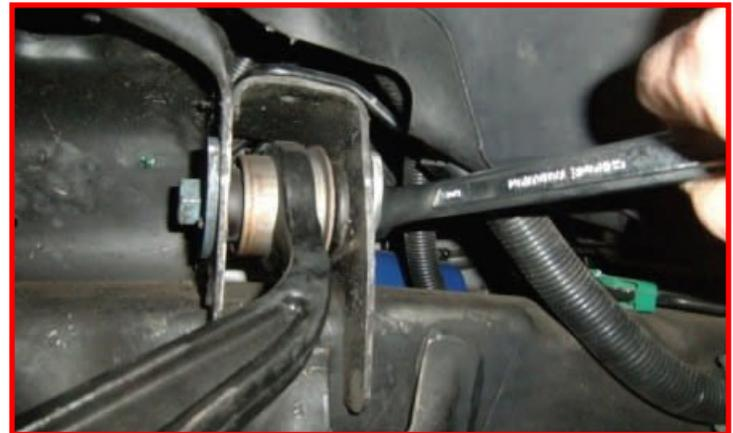
Remove the upper control arm from the frame rail.
