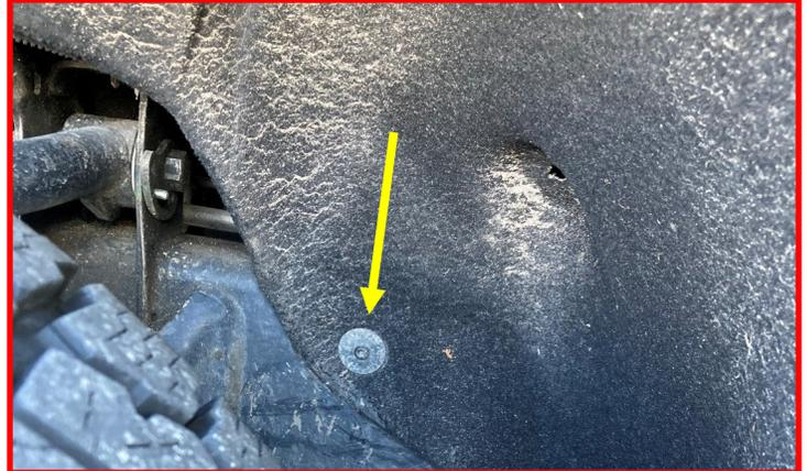
Install the fender liner using the two previously removed screws.
