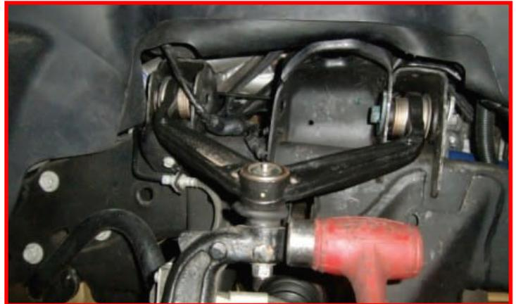
Remove the upper control arm bolts from the frame rails. Mark the cam bolt and cam orientation for re-installation.
