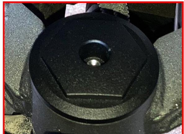
Install Falcon front shock using supplied hardware on top and factory hardware on the bottom.
