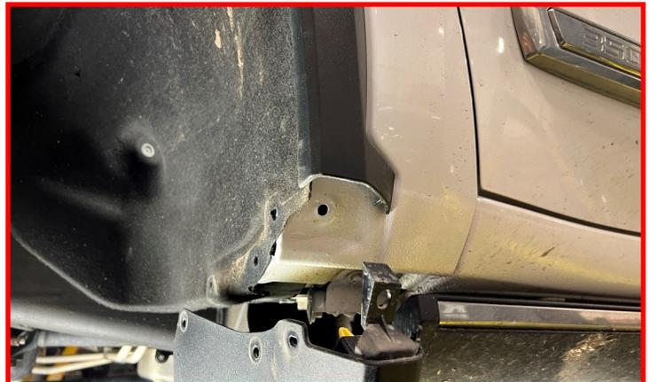
Remove the two screws holding the fender liner to the inner fender well and carefully pull the liner out from under the fender flare.
