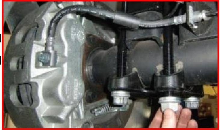
Trim off excess u-bolt length with a suitable cutting tool if desired.
