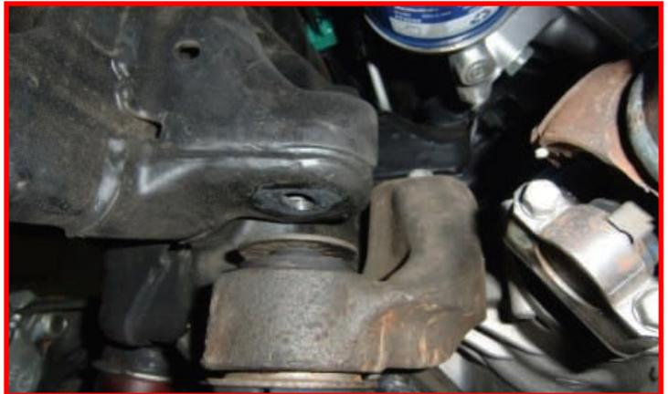
Install the 1/2" ReadyLIFT differential spacers between the frame and differential cradle. Use the provided laser cut washers and M14x130 bolts, reuse factory flange nuts.
