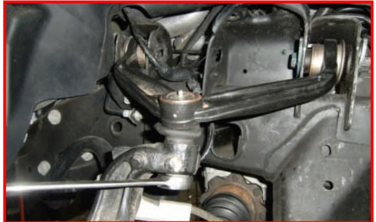
Strike the ball joint boss with a dead blow hammer to dislodge the taper.
