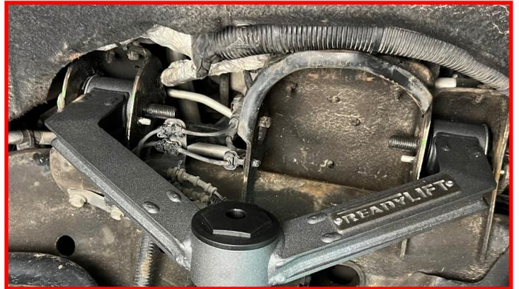
Install the upper control arm ball joint to the factory knuckle using the provided hardware.
