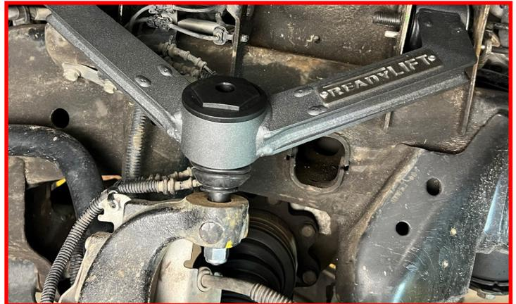
Grease the upper ball joint using a high quality ball joint grease and a needle type grease gun. DO NOT over grease.
