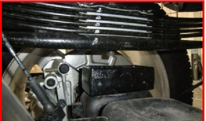
Raise the axle with the ReadyLIFT block installed to the leaf pack. Install the provided U-bolts and hardware. Ensure the lock washer is located between the nut and thick washer. Only snug the U-bolts up enough to hold the axle in place. Repeat all steps on the passenger side. Final torque will be done when the vehicle is on the ground.
