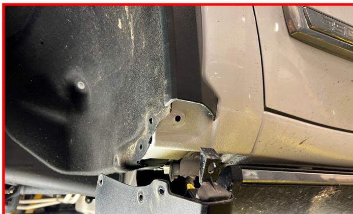
Remove the two screws holding the fender liner to the inner fender well and carefully pull the liner out from under the fender flare.
