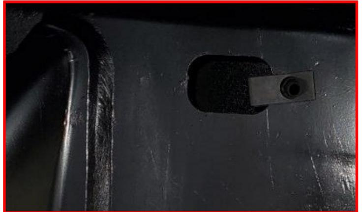
Attach the fender liner using the 1/4 fender washer and thread cutting bolt.
