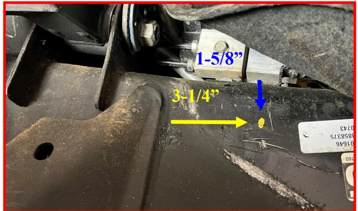
Debur the hole and coat with some type of anti-corrosion coating such as undercoating or paint.
