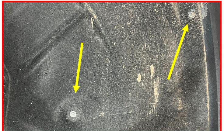
Remove the outer most rear tab on the factory mud flap.
