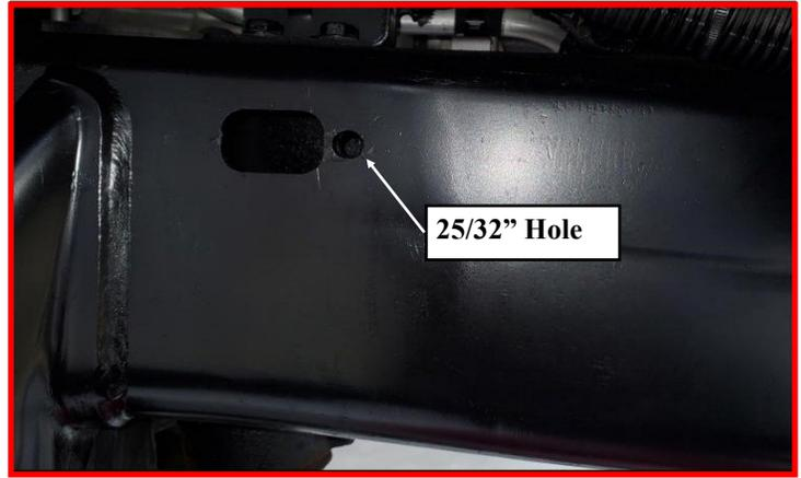
On vehicles lacking the slot in the frame just behind the weld securing the cross member:
