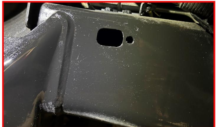
Press the fender liner towards the new hole and drill a 1/4" hole in the liner.
