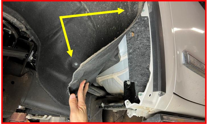
Remove the three bolts securing the black bracket.
