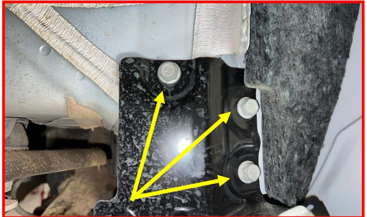
Remove the u-nuts from the black bracket and install them on the new fender bracket.
