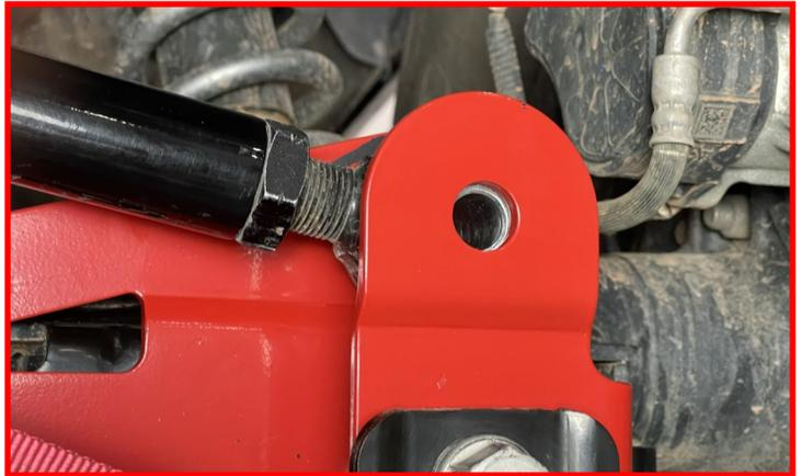
Torque the factory bolt to 120 ft.-lbs.
