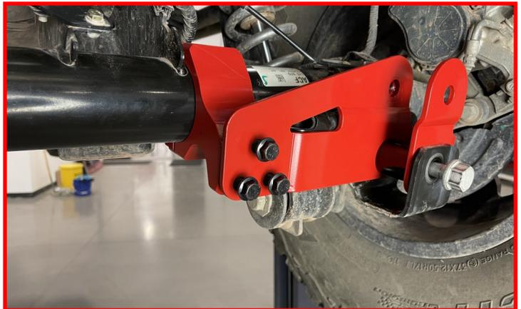
Install the (6) **M8-1.25 x 25mm socket cap screws** through the **rear track bar clamp** and into the **front track bar clamp**.
