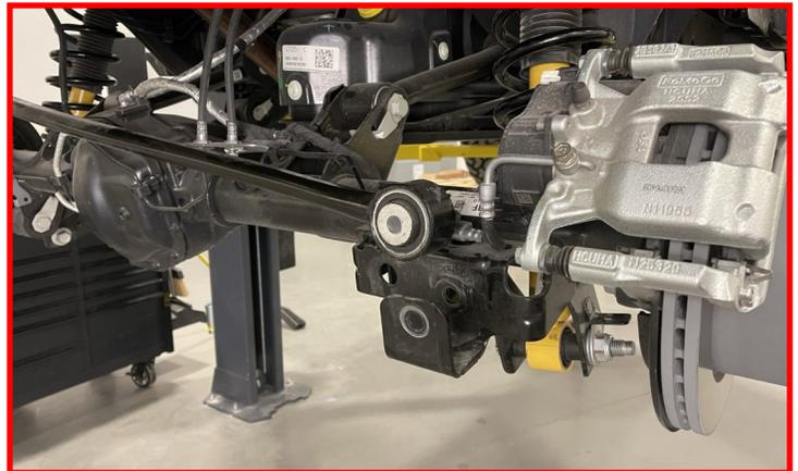
Install the supplied **rear track bar bracket** in the factory location using the supplied **rear track bar bracket spacer** and the factory track bar axle pivot bolt.
