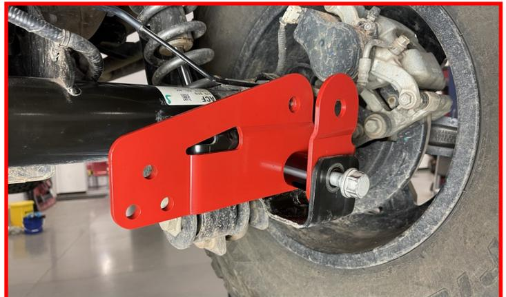
Install the **front track bar clamp** on to the axle.
