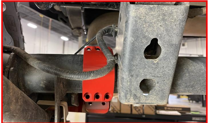
Align the (3) mounting hole on the track bar bracket to the **front track bar clamp**.
