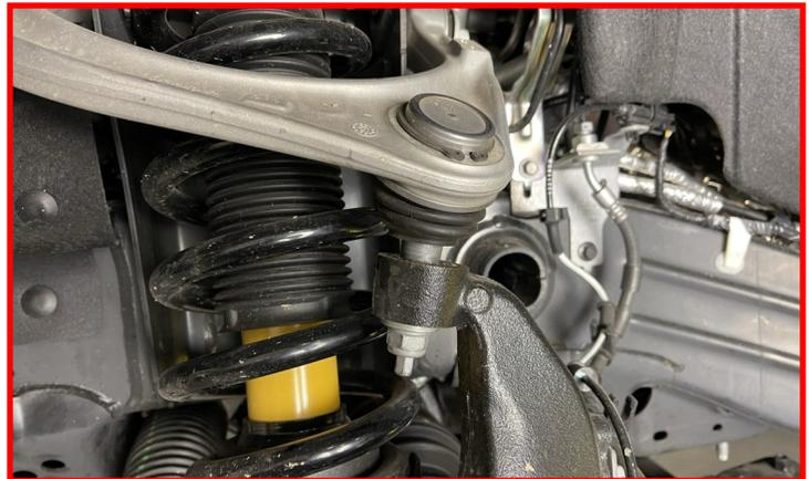
Remove the upper control arm pivot bolt.
