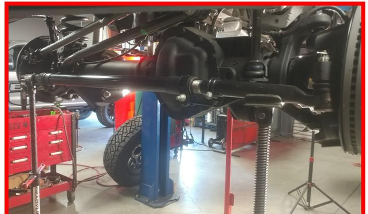
Remove the factory radius arm pivot hardware.
