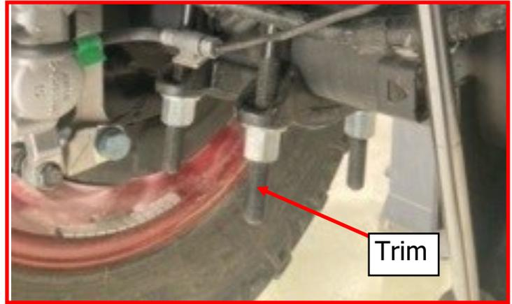
Jounce the vehicle to settle the suspension to the new ride height. Torque the radius arm hardware to **225 ft-lbs** and shock hardware to **65 ft-lbs**.
