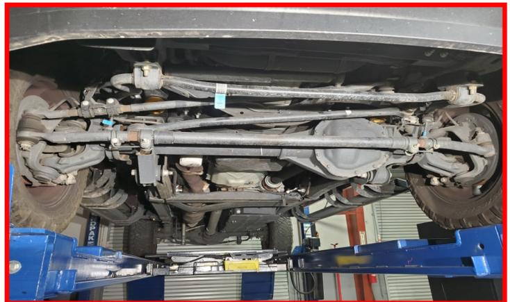
Remove the (2) middle bolts on the passenger side of the differential cover and retain the factory hardware. Remove the differential ID tag and either place in a secure location (skip next step), or reinstall on the driver side of the differential (see next step).
