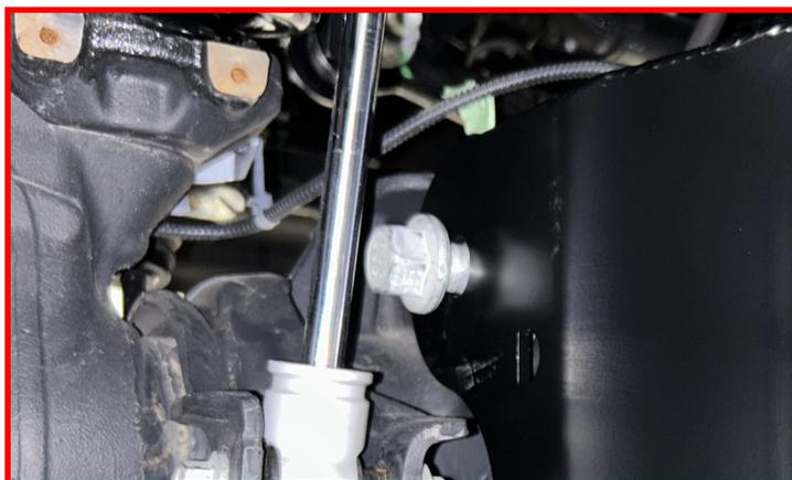
Install the track bar into the track bar bracket using factory hardware.
