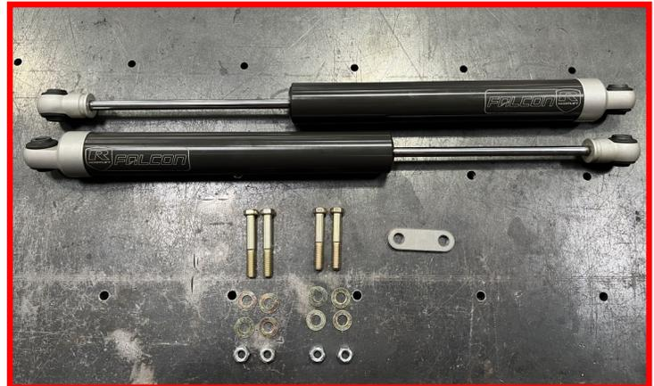
Using the **M12 x 75mm bolts, washers and nuts**, install the body end of the stabilizers onto the center stabilizer bracket. Stabilizer body end should be installed with the **stabilizer top plate** on top and the **center stabilizer bracket** on bottom (as shown in photo). Do not tighten at this time.
