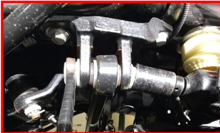
Remove the cast track bar mount on driver side of frame.
