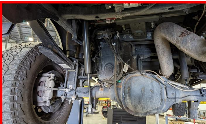
If equipped with a 2 piece driveline, remove the bolts holding the carrier bearing to the frame. Install the ReadyLIFT carrier bearing spacer between the carrier bearing and frame using **7/16" bolts, washers and nuts**.
