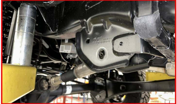
Install the replacement radius arm to axle using factory hardware for the upper connection and using the supplied cam bolts for the lower connection.
