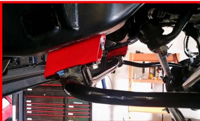
Install the **brake line drop bracket** to the original hole in the frame rail using the factory bolt.
