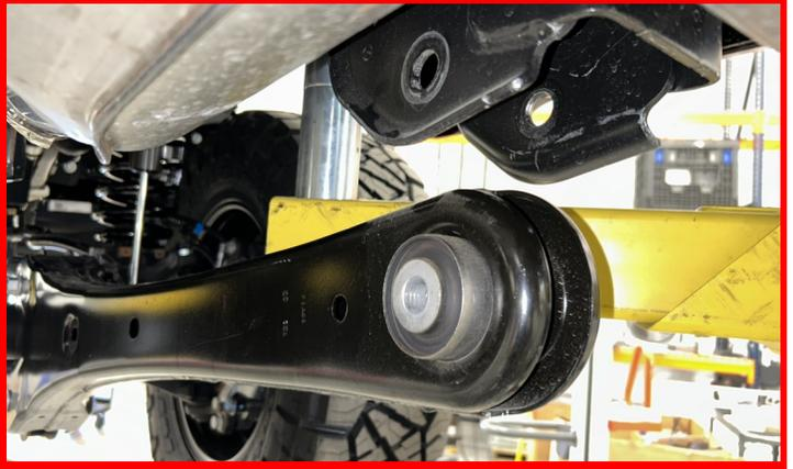
Remove the (2) radius arm axle mounting bolts.
