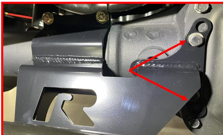
Using the supplied M10-1.5 x 55mm Hex Head Bolts, M10 flat washers and M10-1.5 toplock nuts, fasten the rear axle bracket to the center stabilizer bracket, clamping both around the axle tube.
