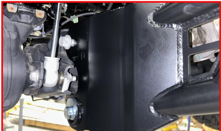
Carefully raise the radius arm into the drop bracket and secure it using the factory hardware.
