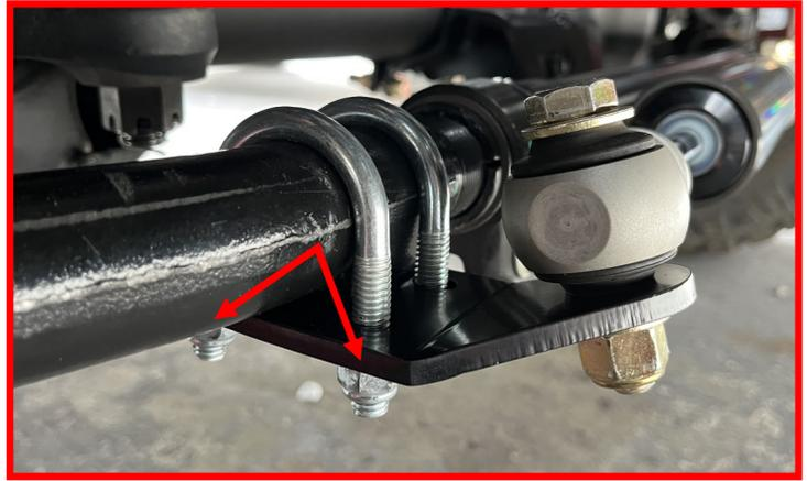
Space each tie rod bracket an equal distance from the center bracket. When in the correct position, tighten the nuts.
