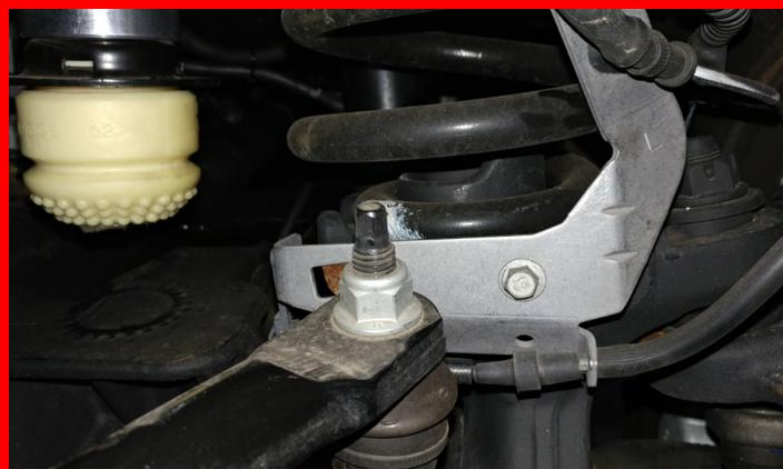
Remove the factory bump stop by pulling it out of its mount. Remove the mount from the frame.
