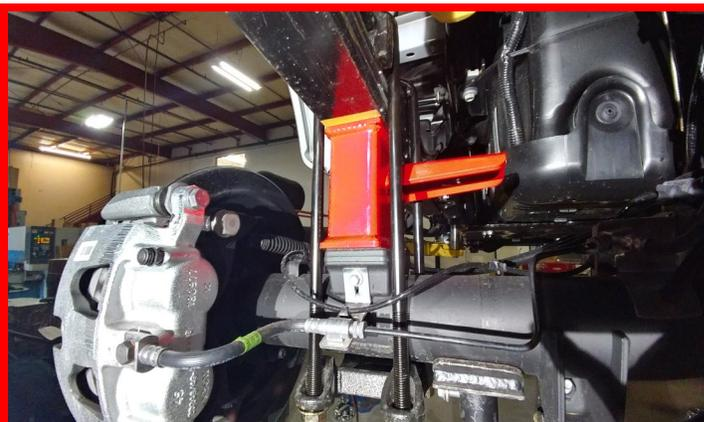
Install rear Falcon shock using factory hardware.
