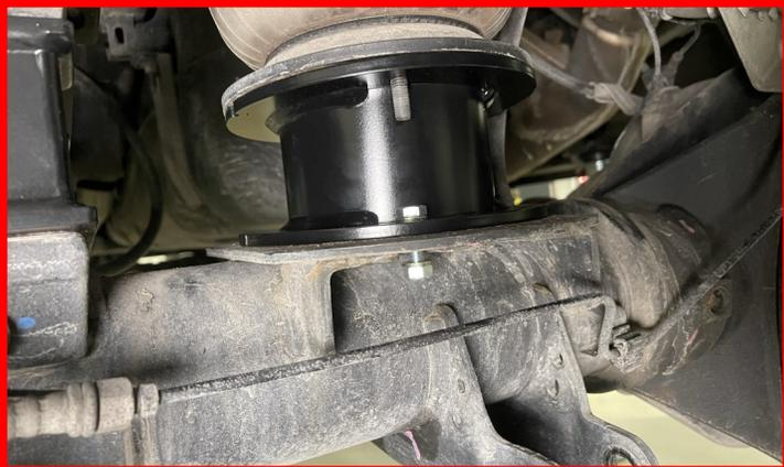
Install the factory air bag mounting nut on to the air bag.
