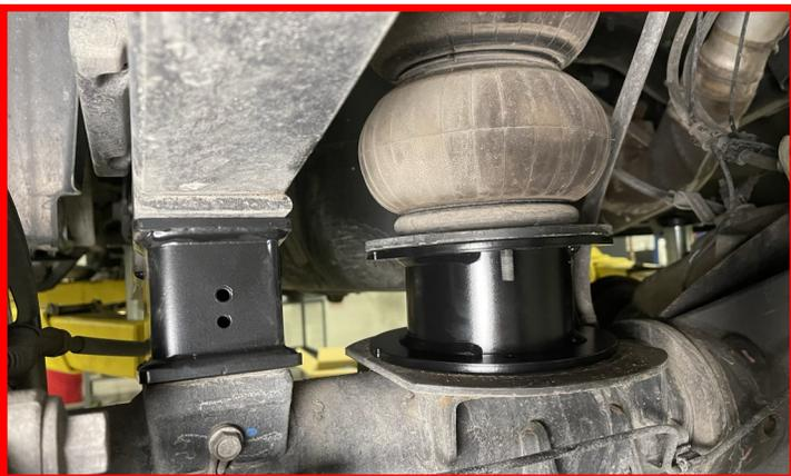
Mount the rear air bag spacers to the axle using the supplied M8 x 30mm, M8 flat washers and locking nuts.
