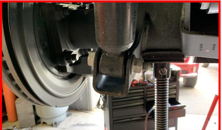
Remove the factory air bag lower mounting nuts.
