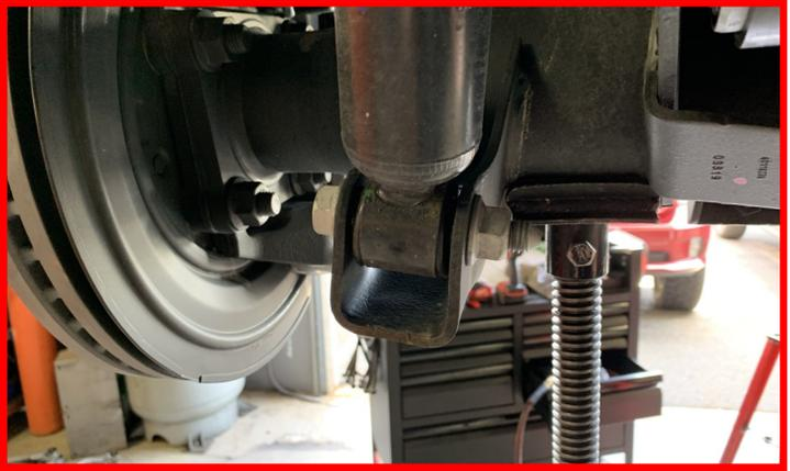
Plug the factory air suspension height sensors in.
