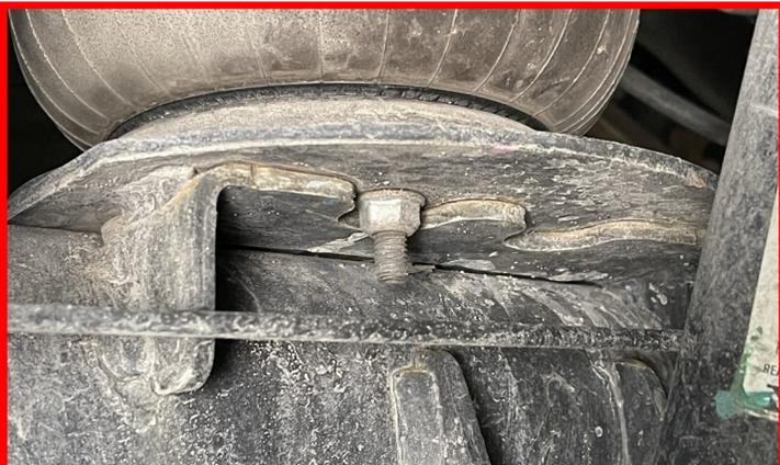
Lower the axle enough to allow the rear air bag spacer to be installed.
