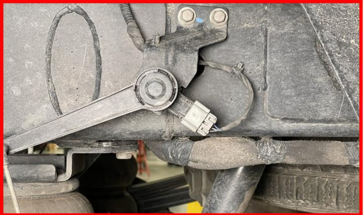
Install the rear wheels. Lower the vehicle to the ground. Torque the lug nuts to the wheel manufacturers specs. Torque the lower rear shock hardware to **90 ft-lbs.** Connect the vehicle power source at the ground terminal on the battery. Check to make sure that your air system functions properly.
