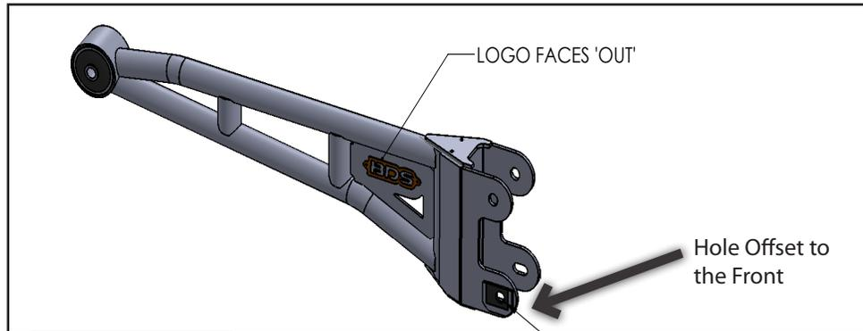
29. Tighten the front hardware at the axle to 222 ft-lbs. Do not tighten the frame pivot hardware at this time.
