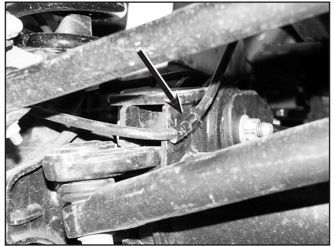
9. Disconnect the sway bar end links from the sway bar. Retain hardware.
