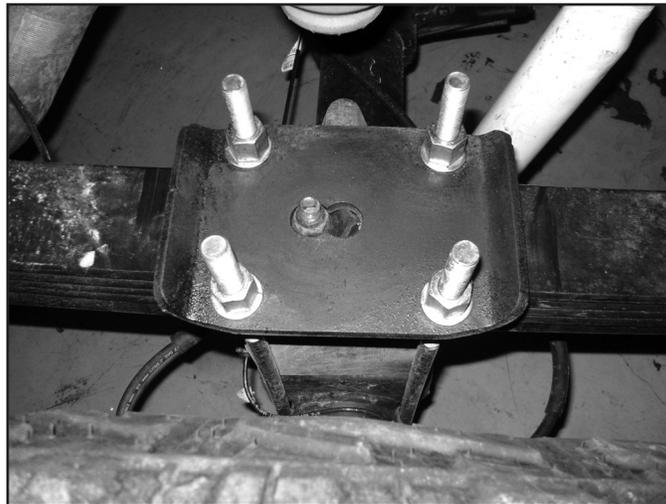
57. Repeat block installation of the driver's side. Take care not to over extend the brake lines.
