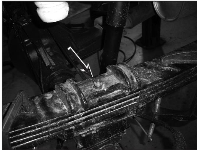
54. Remove the factory lift block. It will not be reused.
