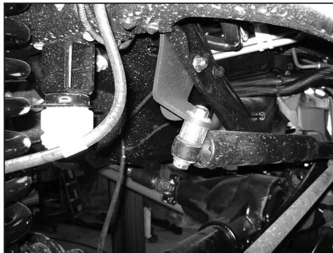
14. Disconnect the (5) bolts mounting the OE track bar bracket to the frame. Remove bracket and retain hardware.
