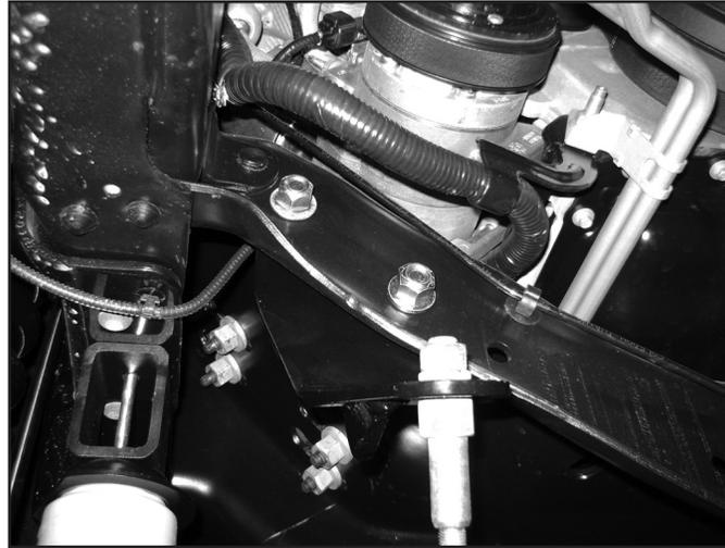
13. Position the stabilizer under the new bracket and install with the provided 12mm hardware (Bolt Pack 657) and 3/4" steel spacer (YJTC5). (Fig 7) Torque to 50 ft-lbs.
