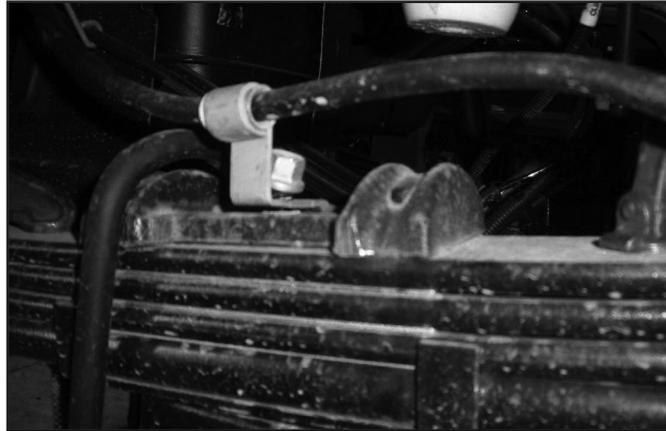
64. If more parking brake cable slack is needed, remove the cable from the rear-most retaining bracket on the frame. (Fig 21)
