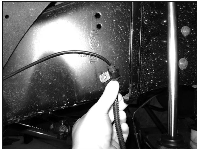
40. If needed, attach ABS wires to the radius arm with the included zip ties and push pin zip tie where the upper mount at the axle is located. Allow axle to droop out to check for adequate slack.
