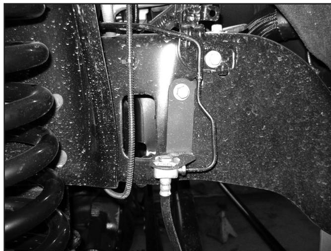
43. Properly bleed the brake system of air and top off the brake fluid reservoir with the proper type of fluid (see owners manual).
