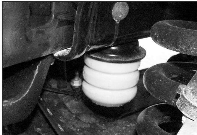
24. Position the cup on the provided bump stop extension. (01001) The alignment tab on the bump stop cup will fit in the second hole in the extension.
