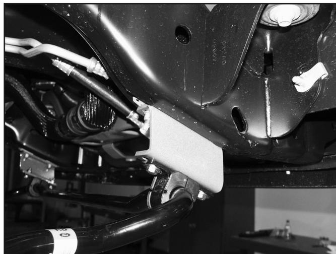
37. Install the sway bar link ends to the sway bar and secure with the OE hardware. Torque to 90 ft-lbs.
