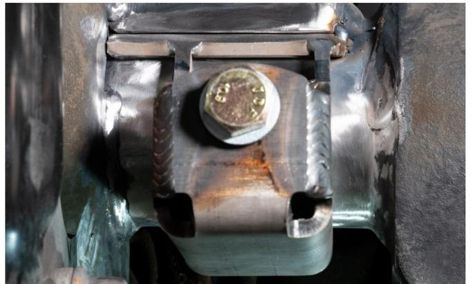
5. With the shock mount in place, weld the shock mount to the axle tube.
