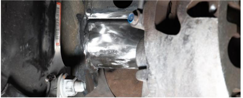
3. Grind a taper into the arced surface to prep it for installation to the axle tube.
