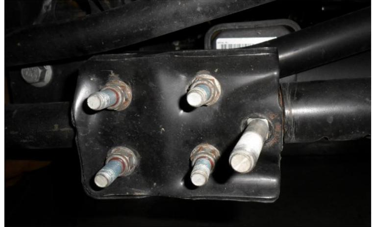
5. Tighten the U-bolts on factory stabilizer clamp to 45 lbs/ft and make sure the bracket is facing straight out. Install the 2 gold spacers from the Hardware kit onto the stud, then place the Body end of the shock onto the stud, one more gold spacer, then install factory nut. Tighten nut to 30 lbs/ft.
