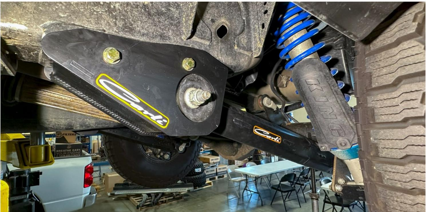
7. Repeat this installation on the passenger side. The removal of the frame-side bolt on the passenger side is impeded by the fuel tank. If you loosen the fuel tank straps (use an 18mm socket), you can slide something (we used a dead-blow hammer) between the frame and fuel tank to scoot it over enough to clear the bolt. Other than this, installation is exactly the same, just mirrored.
