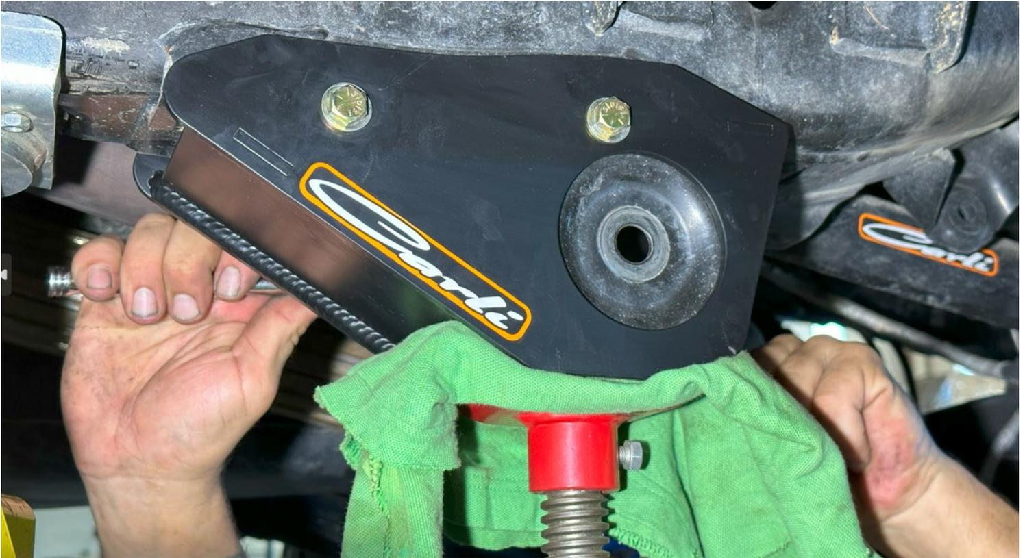
6. Install the control arms (loosely) with the factory hardware.
