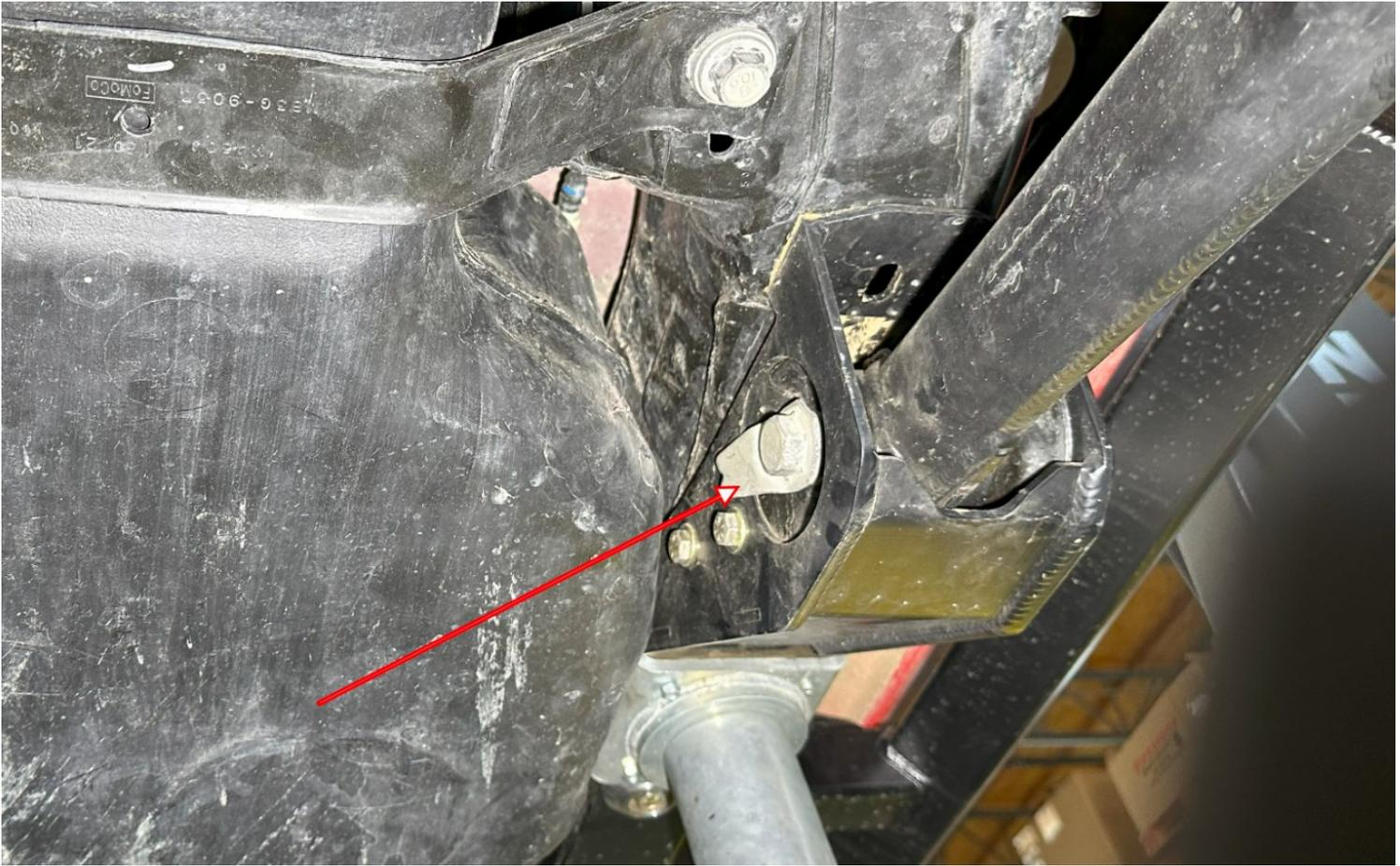
8. **24MM** — The Carli Arms are built with 17-4 Stainless Spherical Joints, The hardware can be torqued at any position; there's no need to torque at ride height. If you're re-installing the factory arms (or any arm with a vulcanized bushing), the Bronco will need to be at ride height when torquing. Torque all factory control arm mounting hardware to 230lb.ft.
