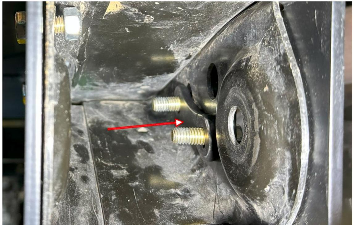
5. **9/16" Socket** — Place a jack under the skid to preload it upward and torque the 3/8" Bolts to 37Lb/ft
