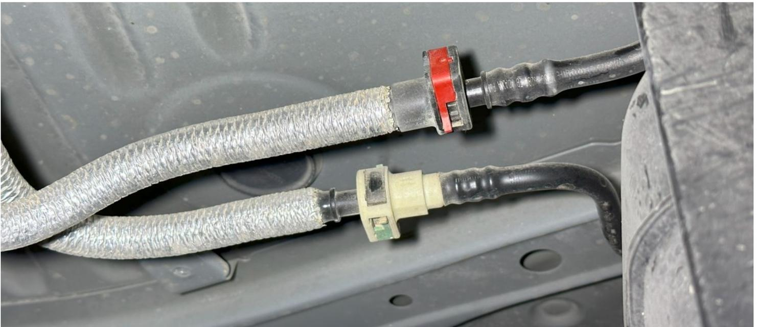
6. Begin lowering the tank while peeking over the top — you'll see the two fuel connections and single electrical connections next to the pickup. Dislodge the fuel lines from the clips that hold them to the top of the tank; this will provide you more room to lower the tank further to access and dislodge the connections. Disconnect the two fuel lines and single electrical connection.
