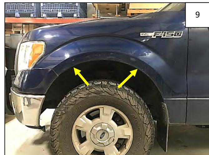
Using a 7/32" socket, reinstall two of the factory bolts through the forward and rearward most holes in the Inner Bracket and into factory holes in fender.
