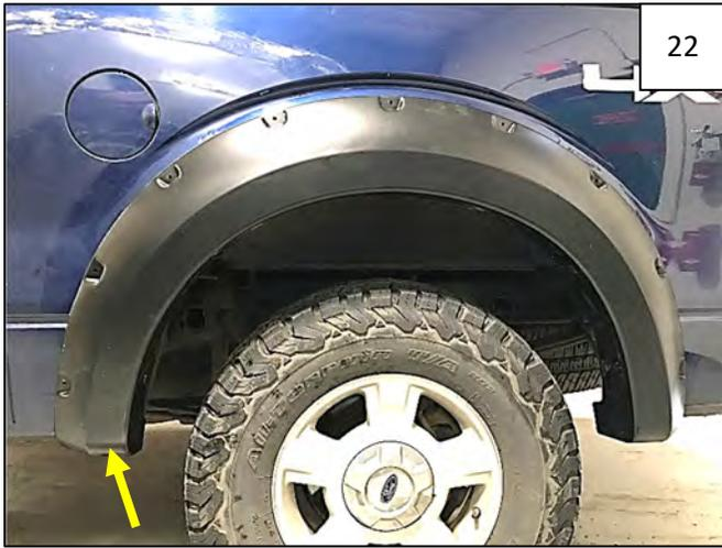
Using a 10mm socket, reinstall foremost factory bolt through flare and into fender.
