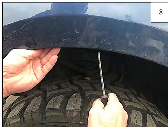
Using a Phillips screwdriver, start a supplied Truss Head Screw through center hole in Inner Bracket and into clip installed in Step 5.
