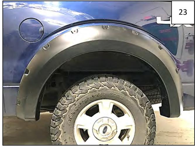
Apply pressure to flare towards vehicle and tighten all fasteners.
