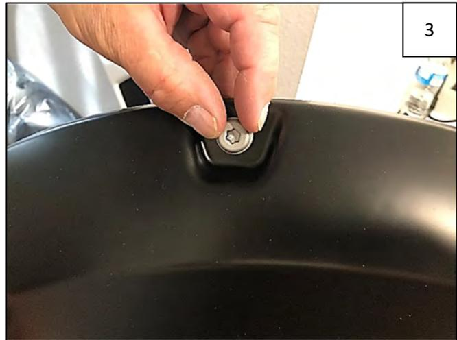
Insert Push-In Pocket Hardware into each flare pocket hole (on outer flare surface, 8 places each front flare, 9 places each rear). Push in to engage clip and tape adhesion.
