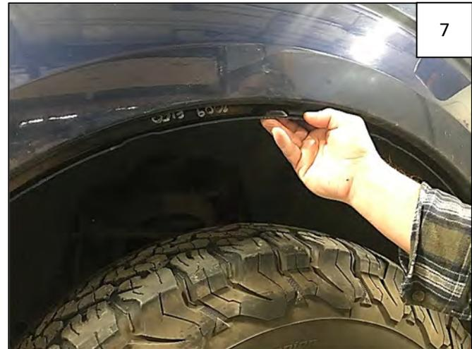
Line up center hole in the Inner Bracket with clip installed in Step 5. NOTE: Driver's side Inner Bracket is marked with an "LF" and the passenger's side Inner Bracket is marked with an "RF".
