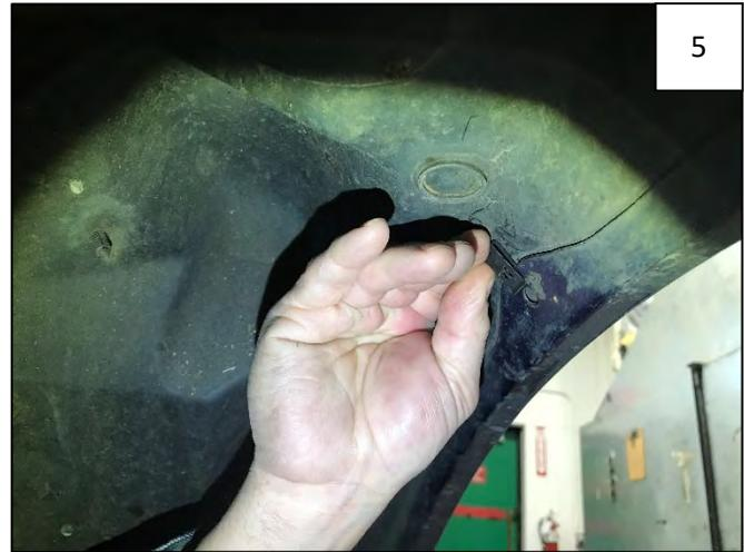
Place a supplied Short "U" Clip over existing factory hole at top of wheel well. Use an awl to center clip over hole.
