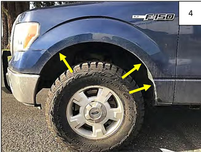
Using a 7/32" socket, remove 3 factory bolts from wheel well. Retain all bolts for reinstallation. NOTE: If you have aftermarket mudflaps, these will need to be removed (and screws retained) prior to flare installation.
