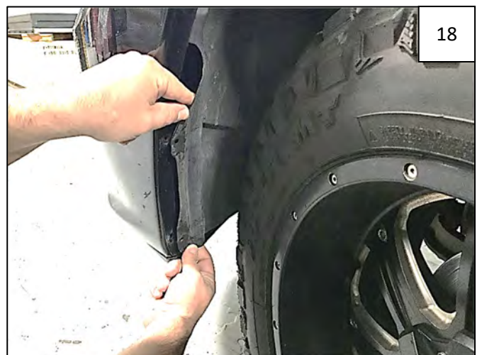
Pull wheel well liner out of lip at front of bumper as shown, exposing 2 factory holes.
