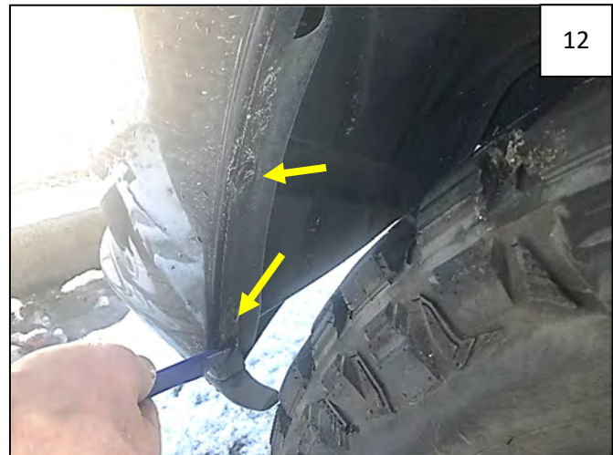
Use a pry tool to disengage and remove two plastic retainers on bumper at front of wheel well.
