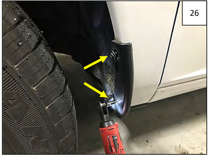
Using an 8mm socket, remove and retain 2 factory fasteners from mud flap.
