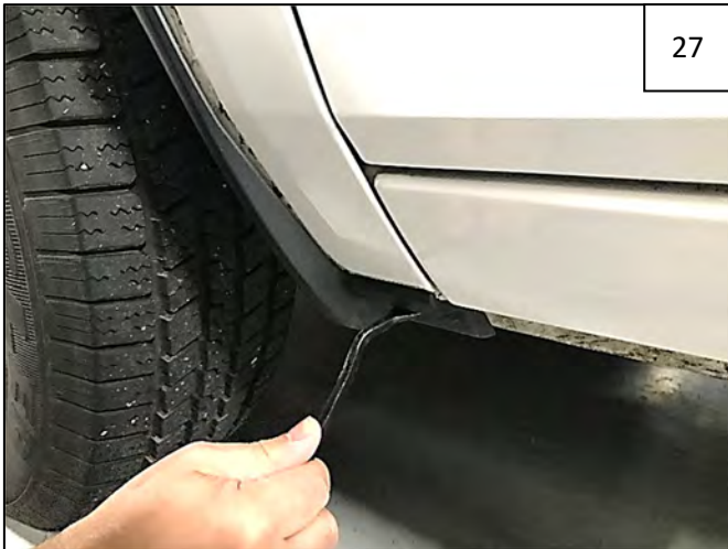
Use a pry tool to disengage plastic retainer at underside of mudflap. Remove and discard mud flap.
