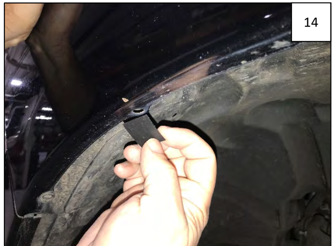
Install a supplied Mounting Tab over factory hole located at top front of wheel well.
