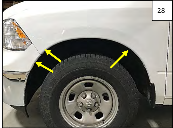
Remove 3 factory fasteners from wheel well at areas indicated by arrows. Retain fasteners for reinstallation.
