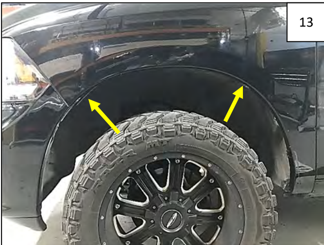
Remove 2 factory fasteners from wheel well at areas indicated by arrows. Retain fasteners for reinstallation.
