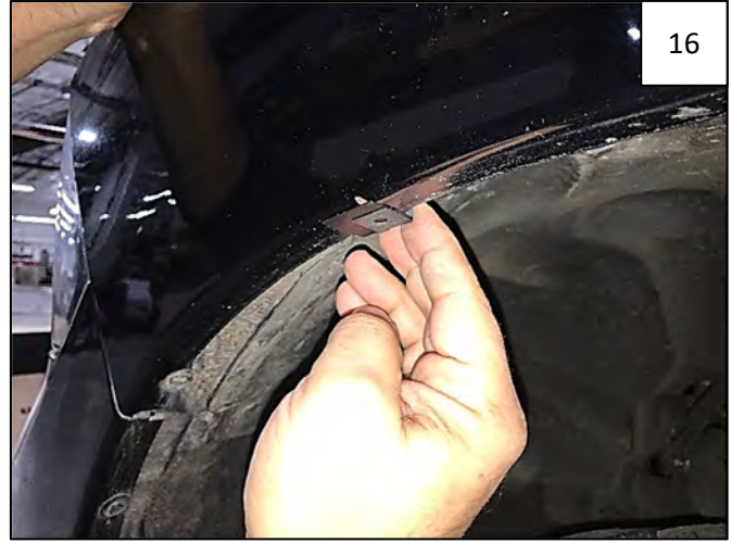
Slide a supplied "U" Clip over tab, centering hole in clip approximately over hole in fender.
