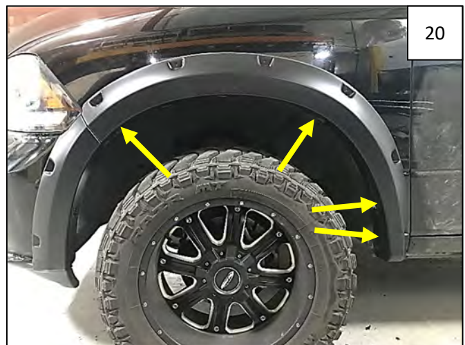
Hold flare on fender and start 4 factory fasteners at locations as shown.
