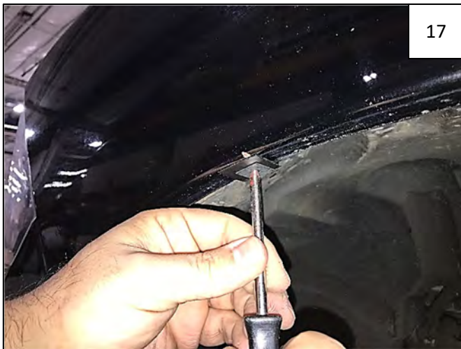
Use an awl to poke a hole in tab for ease of screw installation in Step 21.
