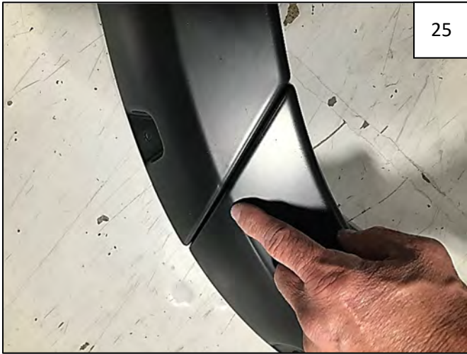
Before tightening, make sure that molded flare features are aligned. Tighten screws using #2 Phillips driver.
