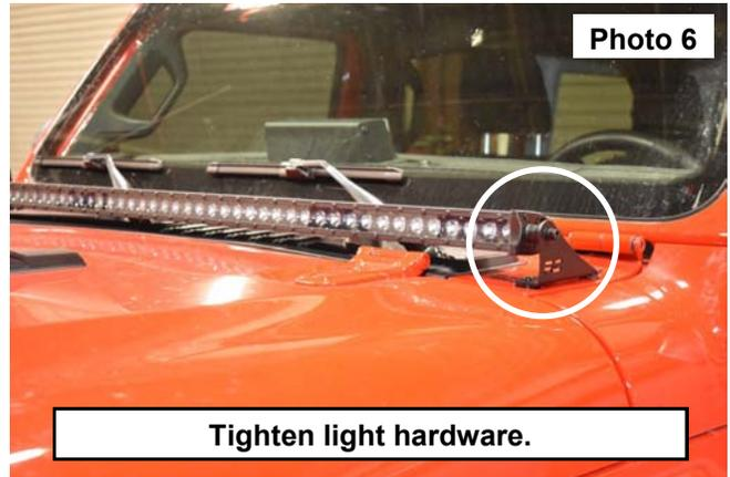
8. At this time follow the instructions supplied with the light to wire the light to the vehicle.
