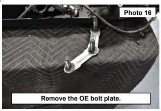
16. Support the bumper. Install the OE bolt plate into the bumper and install the bumper onto the vehicle and secure using the OE retained nuts. See Photos 17 and 18. <u>Pic shown for vehicles without factory receiver hitch. If factory hitch is present, the stock three bolt nut plate will install into the hitch bracket and secure to the bumper.</u>
