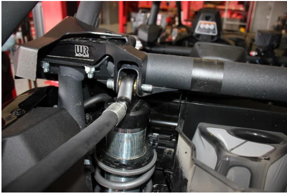
Step 19. Insert the bolt in the top mount, leave loose for now.
