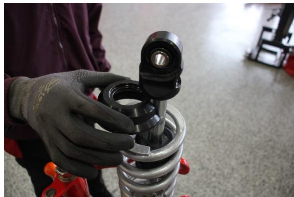
Step 14. Compress spring assembly and re-install spring retainer.
