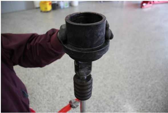
Step 15. Install the OE spring slider.
