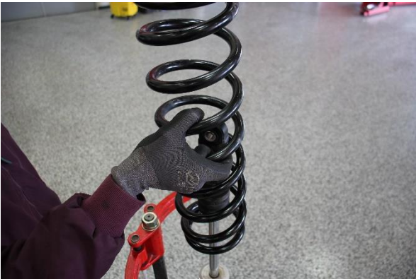
Step 9. Remove OE main spring.
