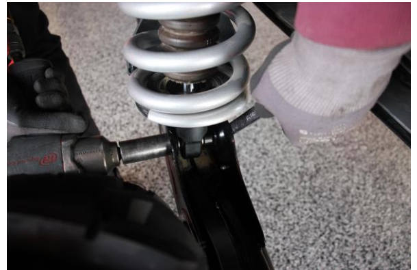
Step 22. Secure the coilover to the control arm with the OE hardware. Tighten upper mount hardware.
