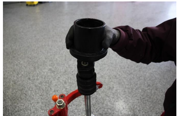
Step 12. Install the OE spring slider.
