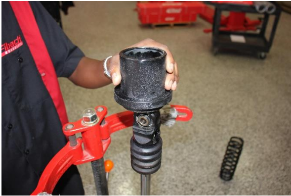
Step 7. Remove OE slider.
