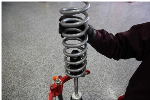
Step 13. Install the Eibach main spring.
