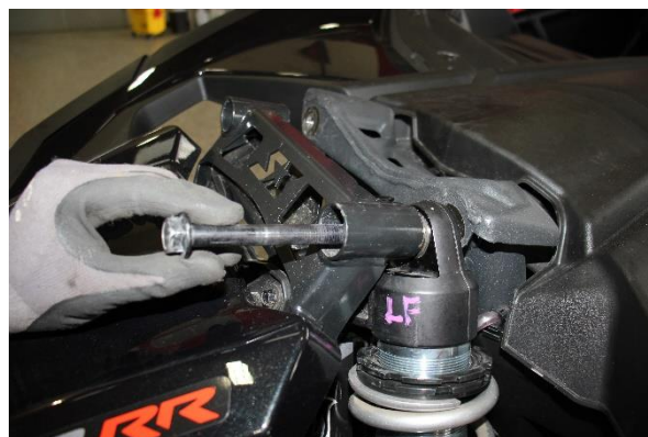
Step 16. Secure the coilover to the upper mount with the OE hardware, leaving loose for now.
