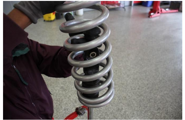
Step 16. Install the Eibach main spring.
