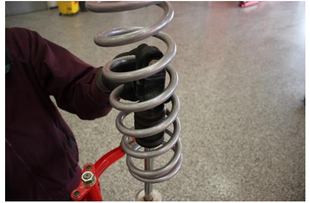
Step 14. Install the Eibach secondary spring.
