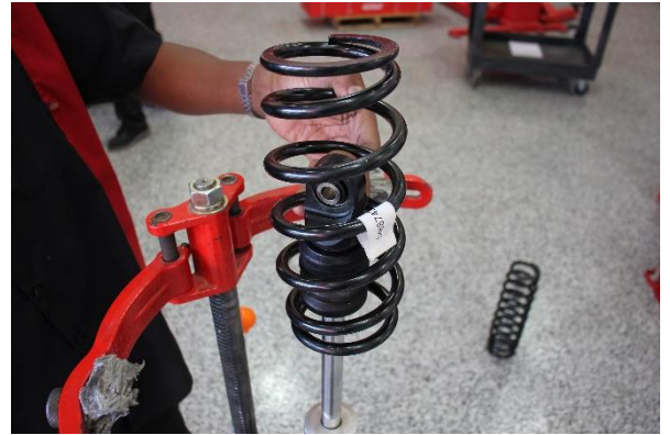
Step 8. Remove OE secondary spring.
