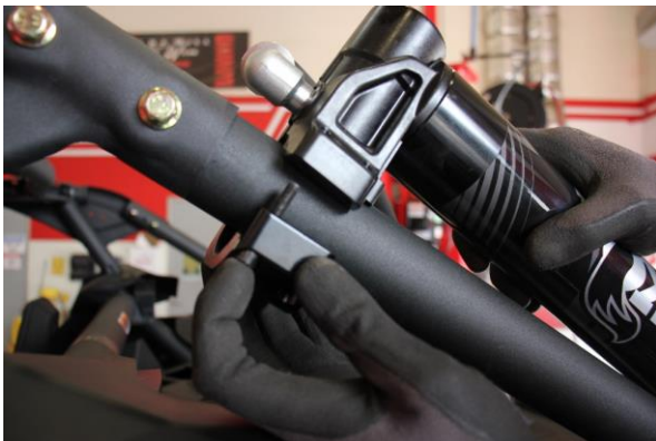
Step 23. Re-install resi one cage, fastened by the 4 socket head cap screws.
