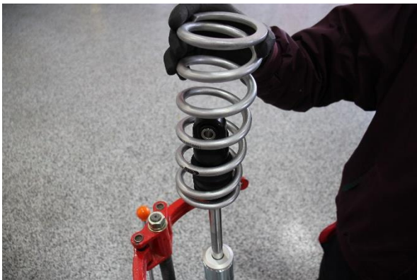
Step 11. Install the Eibach secondary spring.
