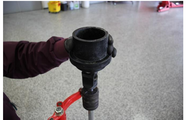
Step 10. Remove OE spring slider.
