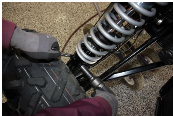
Step 18. Secure the coilover to the control arm with the OE hardware. Tighten the upper mount hardware.
