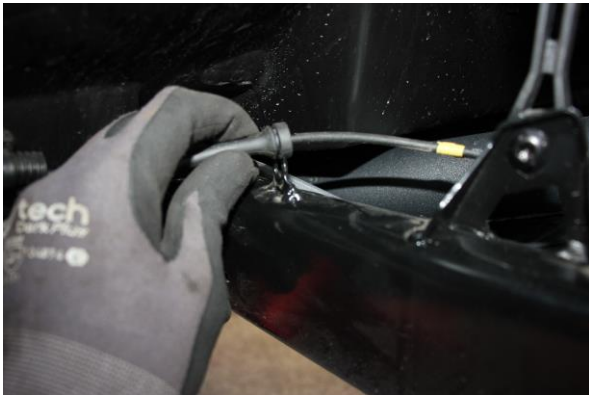
Step 21. Secure the wire to all mounting locations on the control arm.
