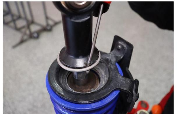
Step 6. Compress the coilover, remove the c-clip. **Note: The bump stop will need to be pried down, out of the way of the spring retainer.**
