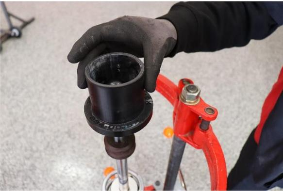
Step 15. Install the Eibach spring slider.
