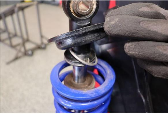
Step 7. Remove spring retainer.
