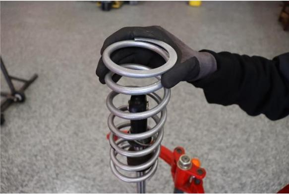
Step 13. Install the Eibach secondary spring.
