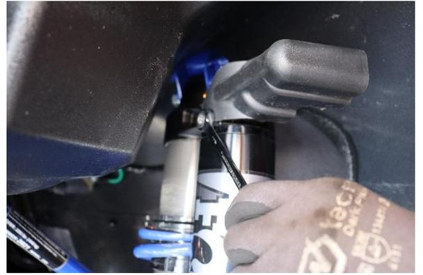
Step 2. Remove electrical connector cover from the top of the coilover.
