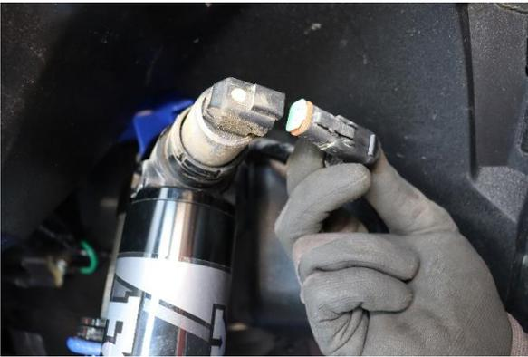
Step 3. Unplug electrical connector from the top of the coilover.
