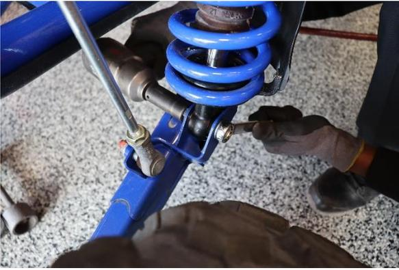
Step 1. Raise the rear of the vehicle and support it with the proper safety equipment. Loosen and remove the hardware that secures the coilover to the control arm. **Note: Never work on or under a vehicle that is not supported by the proper safety equipment.**
