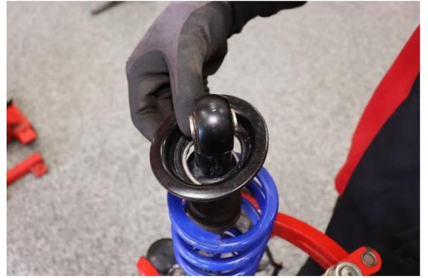
Step 8. Remove spring retainer.
