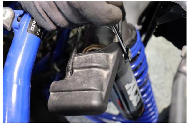
Step 4. Remove electrical connector cover from the top of the coilover.
