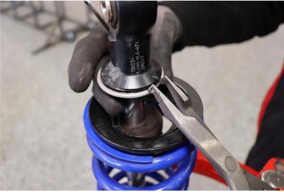
Step 7. Compress the coilover, remove the c-clip .
