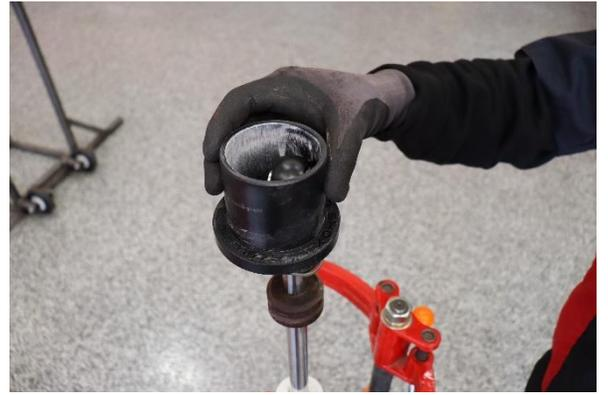
Step 14. Install the Eibach spring slider.
