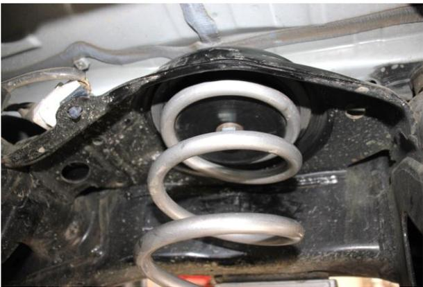
15. Ensure the spring is properly seated on the upper adapter, lower spring seat, and that the urethane adapter is seated correctly on the axle.
