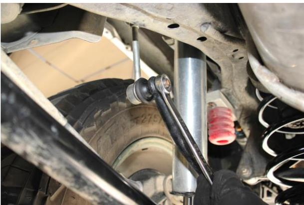
17. Reconnect the end link to the anti-roll bar with the OE hardware as shown.
