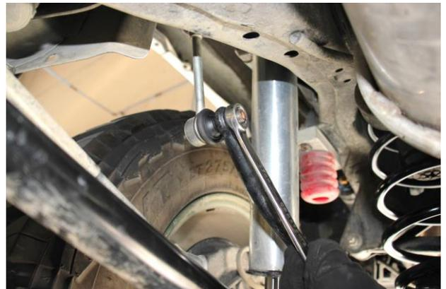
6. Disconnect the end link from the anti-roll bar as shown.
