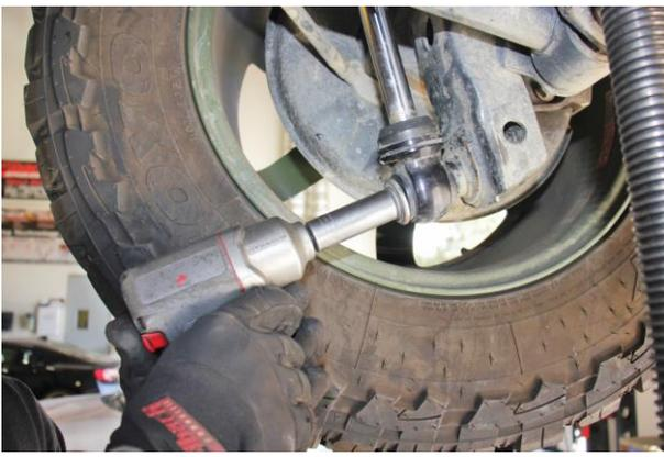
7. Loosen and remove lower shock bolt.
