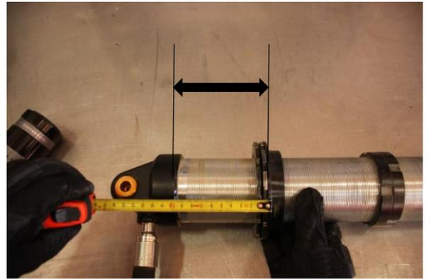
Step 10. Set the preload collar to **100mm** measuring from the base of the reservoir housing to the spring flange.
