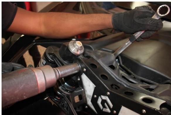
Step 2. Loosen and remove the hardware that secures the coilover to the upper mount.
