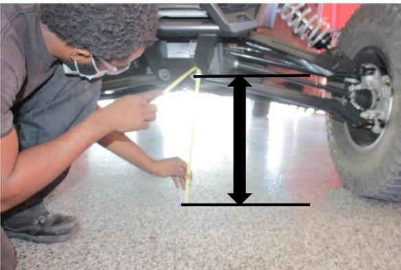
Step 18. Measure from the ground to the center of the lower control arm bolt. The recommended preload measurement in **Step 8** will get the vehicle close to the recommended ride height but each vehicle may vary some. We recommend setting the ride height at **445mm** measuring from the ground to the center of the lower control arm bolt. **Note: If you have larger than stock wheels and tires, the ride height will be increased.**
