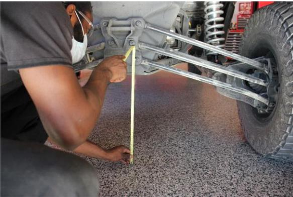
Step 21. Measure from the ground to the center of the lower radius arm bolt. The recommended preload measurement in **Step 10** will get the vehicle close to the recommended ride height but each vehicle may vary some. We recommend setting the ride height at **500mm** measuring from the ground to the center of the lower control arm bolt. **Note: If you have larger than stock wheels and tires, the ride height will be increased.**
