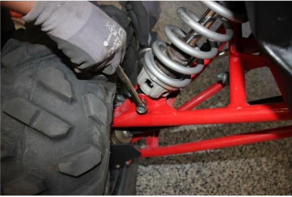
Step 1. Raise the front of the vehicle and support it with the proper safety equipment. Loosen and remove the hardware that secures the coilover to the control arm. **Note: Never work on or under a vehicle that is not supported by the proper safety equipment.**
