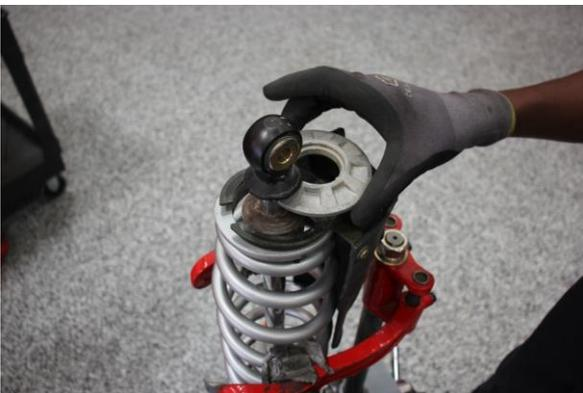
Step 5. Compress the coilover, then remove the spring retainer and rock guard. **Note: The bump stop will need to be pried down, out of the way of the spring retainer.**
